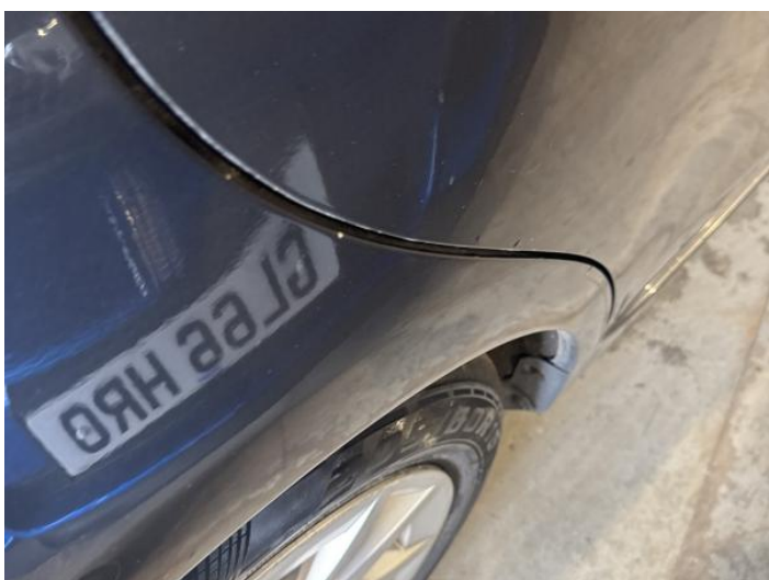
11: Qtr Panel osr Dented 2 Or Less UpTo 10mm
