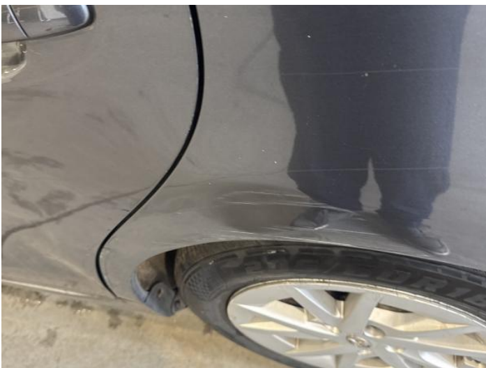
7: Qtr Panel nsr Dented With Paint Damage
