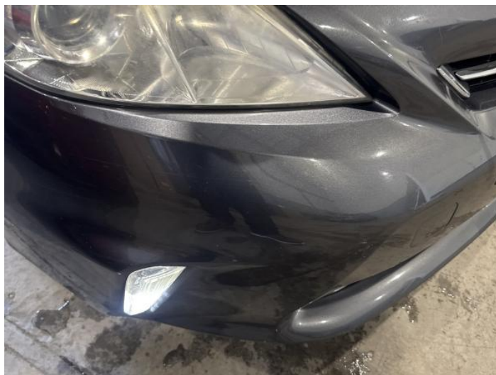
2: Bumper Front Scratched Over 100mm Thru Paint
