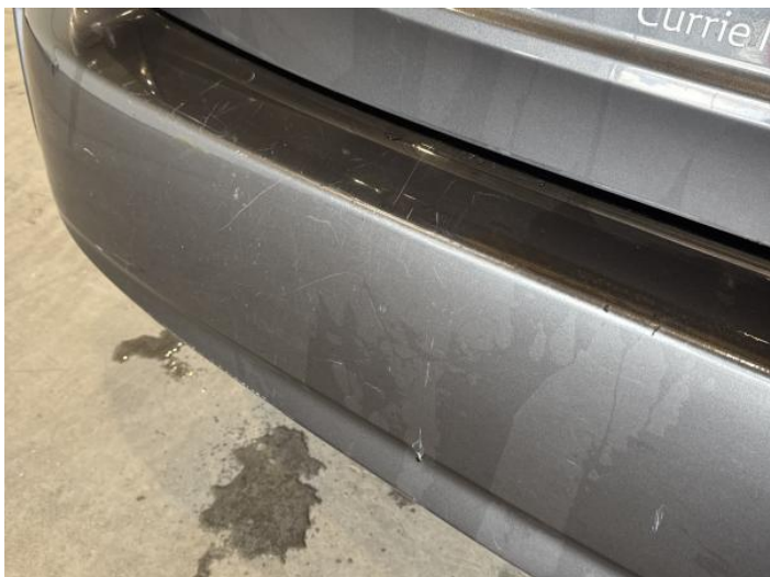
9: Bumper Rear Dented With Paint Damage
