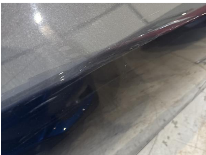
13: Door osr Dented With Paint Damage
