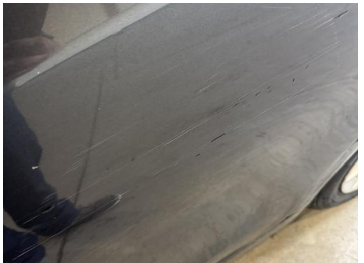
6: Door nsf Dented With Paint Damage
