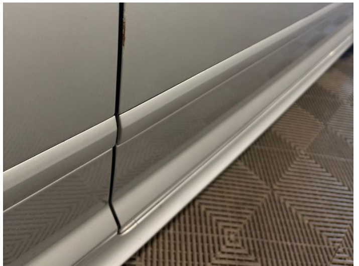
6: Door osf Chipped Edge Chip
