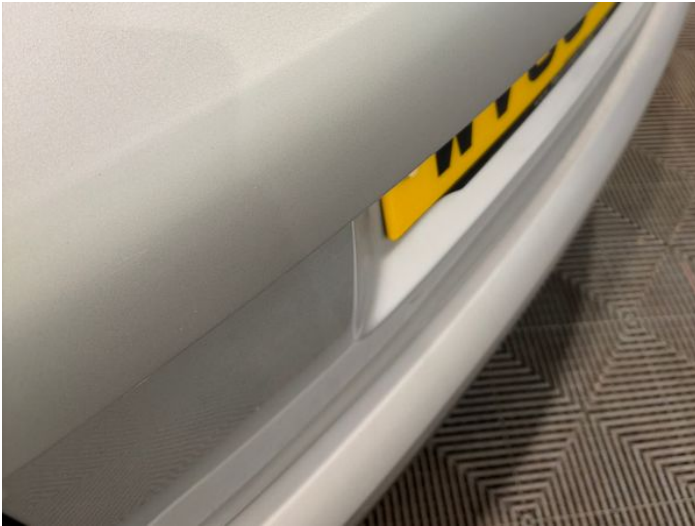
9: Tailgate Poor Previous Repair Poor Paint
