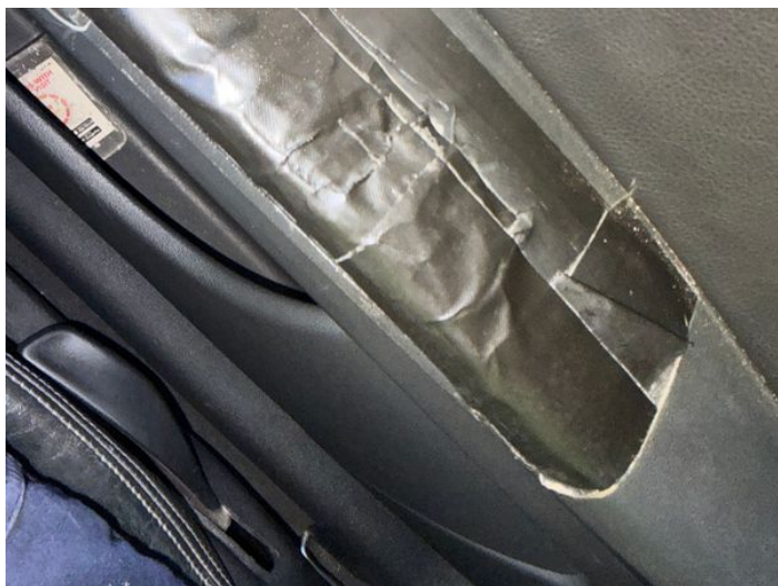
1: Door Pad osf Holed Over 3mm
