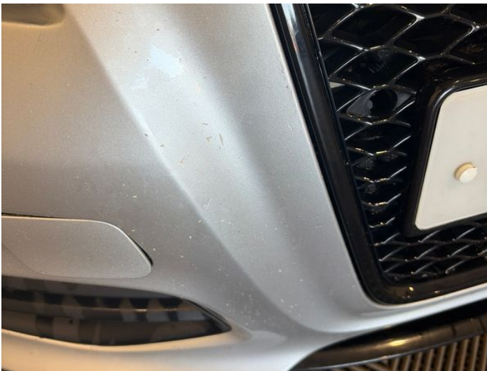
17: Bumper Front Poor Previous Repair Paint Flake
