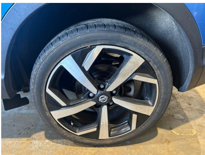
11: Wheel nsr Corroded Light
