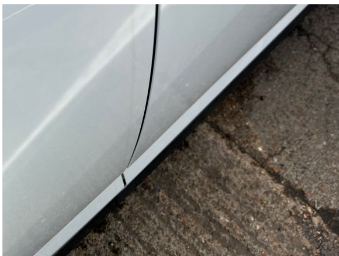
1: Door osf Chipped Edge Chip
