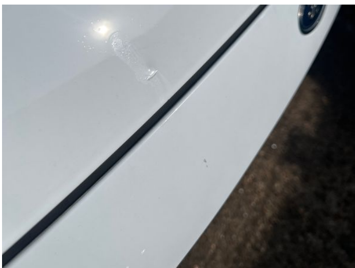
7: Bonnet Dented With Paint Damage
