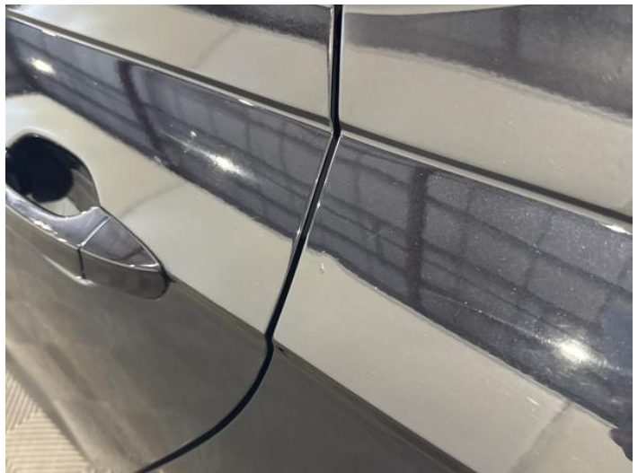
16: Qtr Panel nsr Dented 2 Or Less UpTo 10mm
