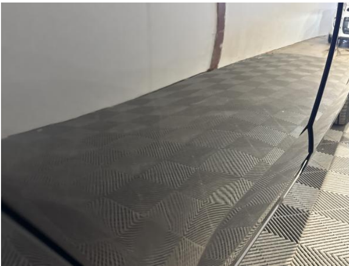
11: Door osr Poor Previous Repair Poor Paint
