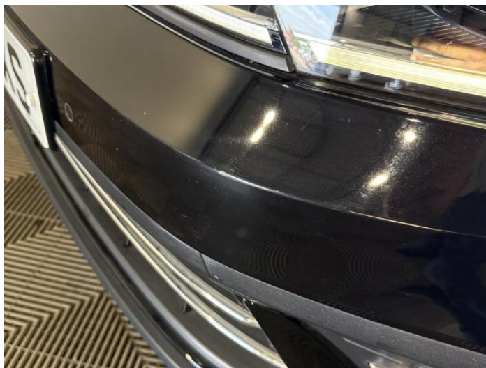
2: Bumper Front Scratched 25 to 100mm Thru Paint
