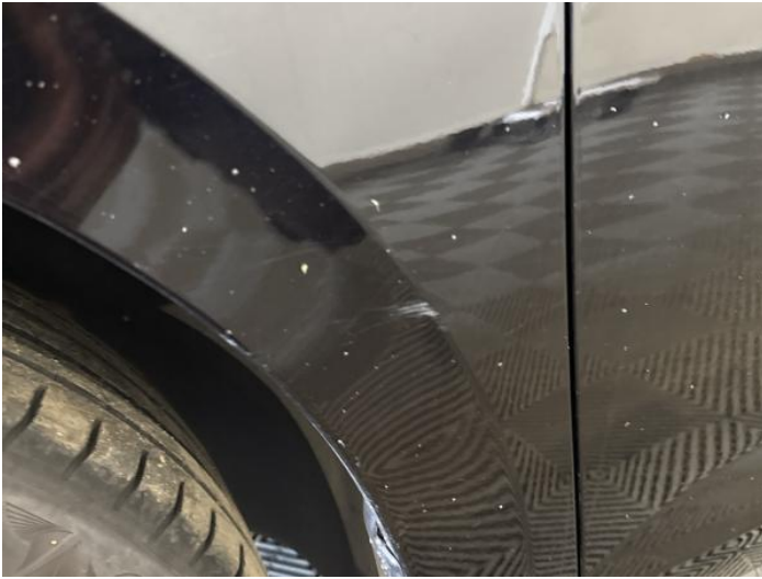
3: Wing nsf Scratched UpTo 25mm Thru Paint
