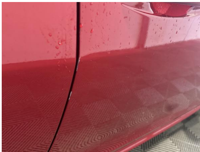
2: Door osf Chipped Edge Chip
