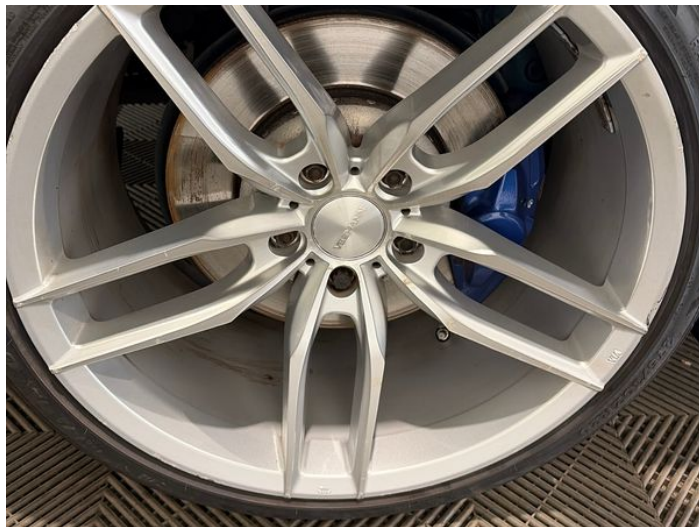
10: Wheel osr Scratched Over 50mm
