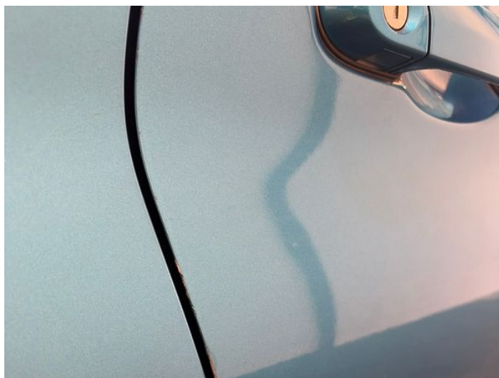
12: Door osf Scratched Over 25mm Thru Paint
