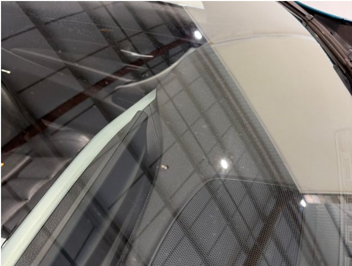
15: Screen Front Chipped Over 10mm
