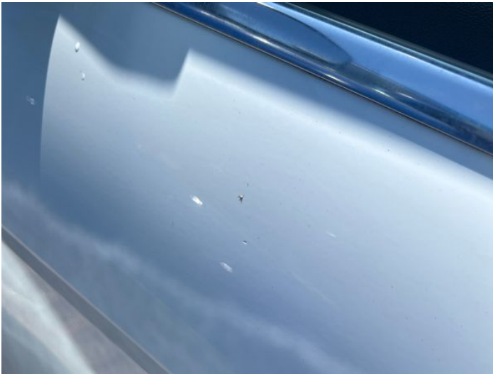
5: Door nsf Chipped 1 To 5
