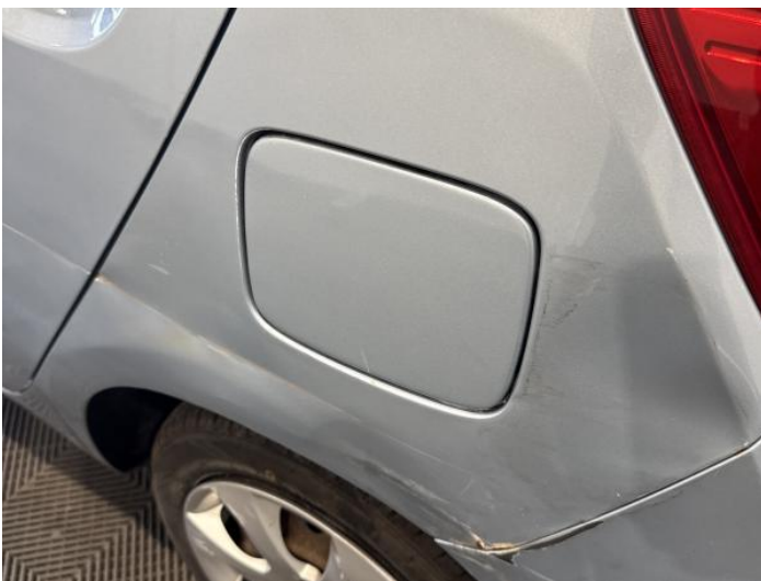
7: Qtr Panel nsr Dented With Paint Damage
