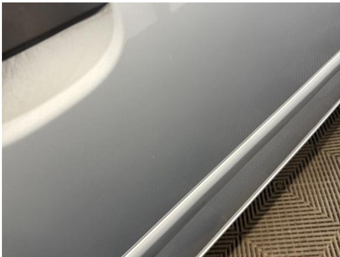
15: Door osf Scratched UpTo 25mm Thru Paint
