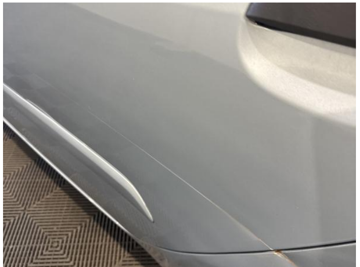
6: Door nsr Dented With Paint Damage
