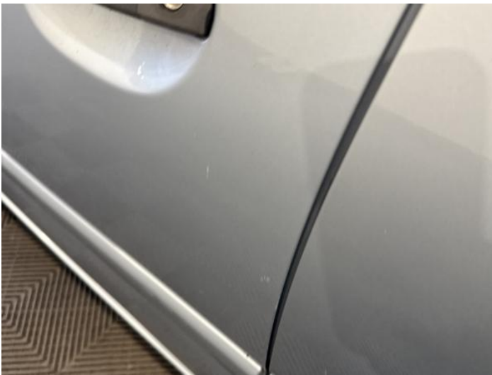
5: Door nsf Scratched UpTo 25mm Thru Paint
