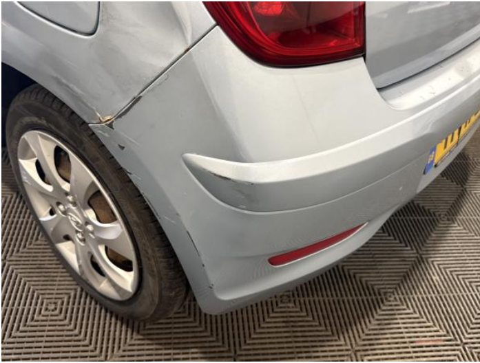
9: Bumper Rear Scratched Over 100mm Thru Paint
