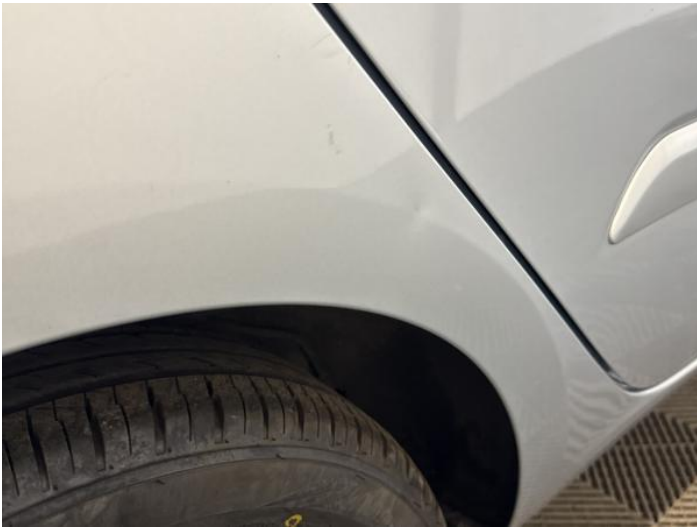
11: Qtr Panel osr Dented Between 10mm + 30mm
