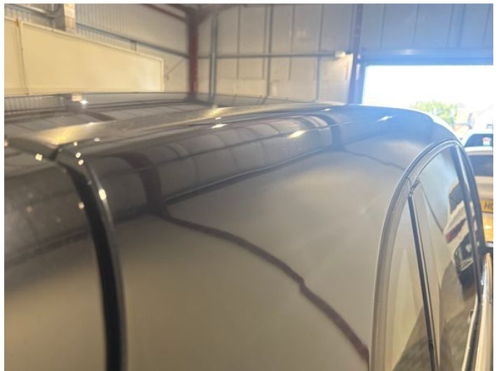
12: Qtr Panel osr Dented Over 30mm
