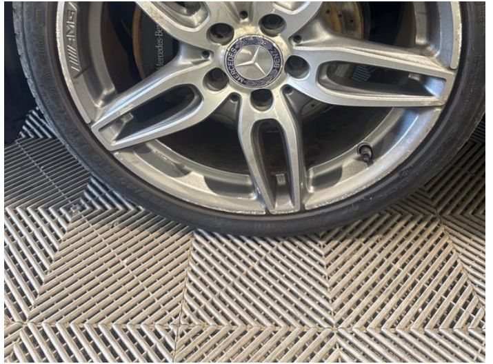
4: Wheel nsf Scratched Over 50mm
