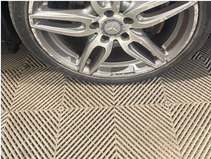
18: Wheel osf Scratched Over 50mm
