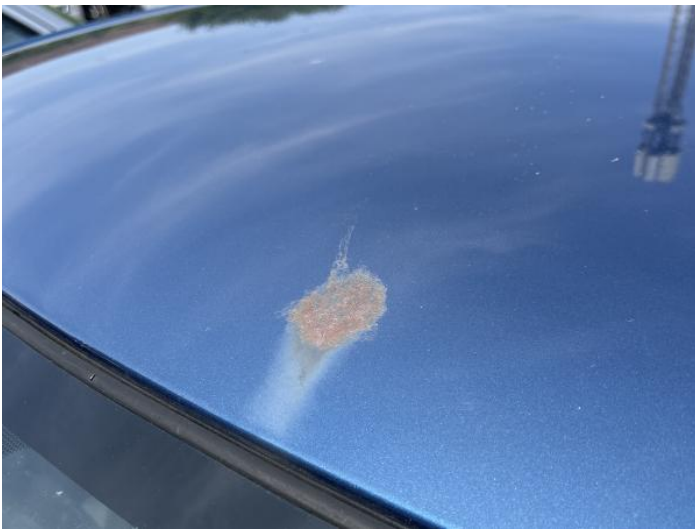
17: Roof Rusted Over 5mm
