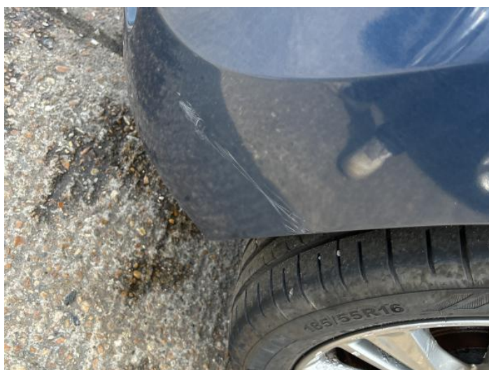
6: Bumper Rear Scratched Over 100mm Thru Paint
