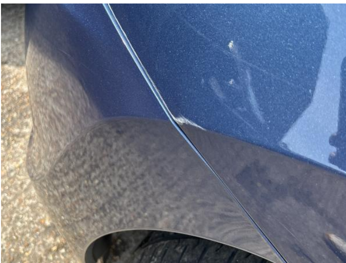
13: Wing nsf Scratched UpTo 25mm Thru Paint
