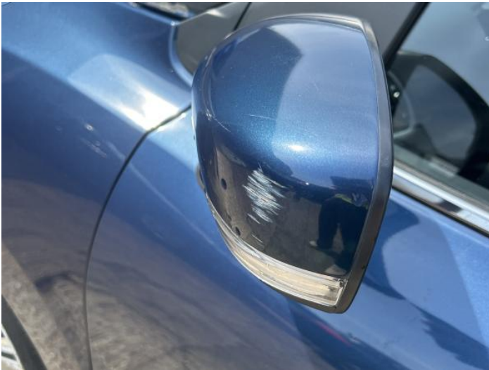
11: Door Mirror Assy nsf Scratched (Painted) Over 25mm Thru Paint
