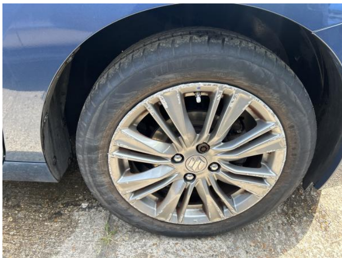
1: Wheel osf Scratched Over 50mm
