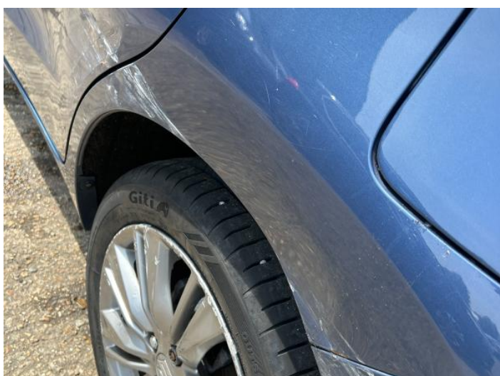
7: Qtr Panel nsr Dented With Paint Damage
