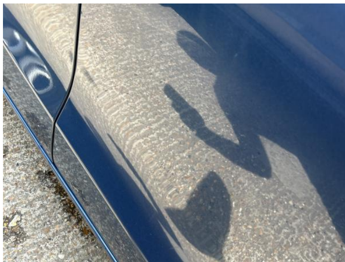
2: Door osf Poor Previous Repair Poor Paint
