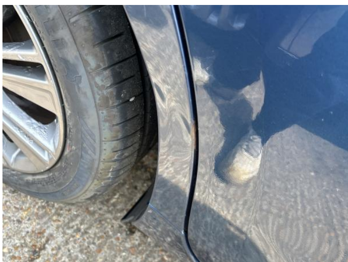
5: Qtr Panel osr Dented With Paint Damage
