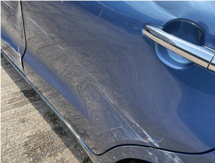
9: Door nsr Dented With Paint Damage
