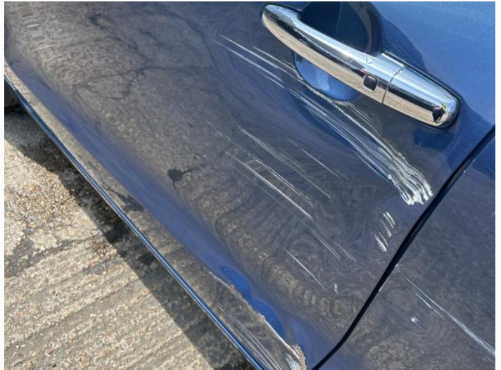
10: Door nsf Dented With Paint Damage
