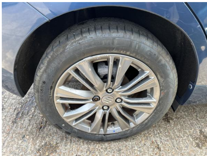
4: Wheel osr Scratched Over 50mm
