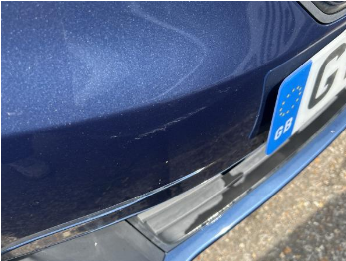
15: Bumper Front Scratched 25 to 100mm Thru Paint
