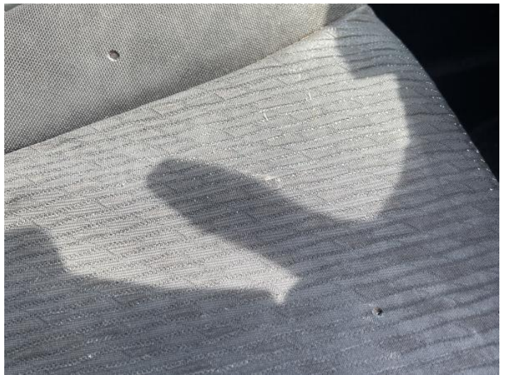
18: Seat Base Cover osf Holed Over 3mm
