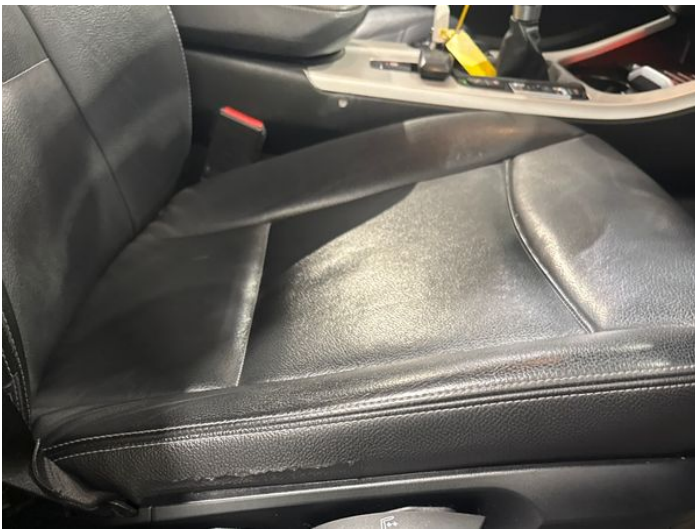
17: Seat Back Cover osf Scuffed Over 25mm
