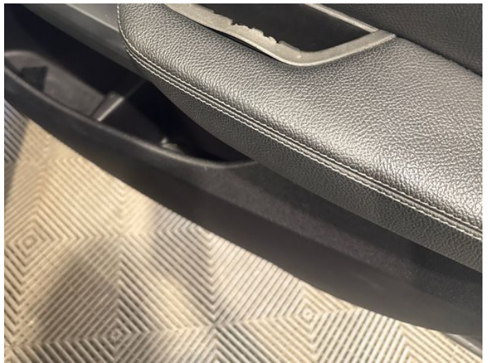
18: Door Pad osf Scuffed Over 25mm
