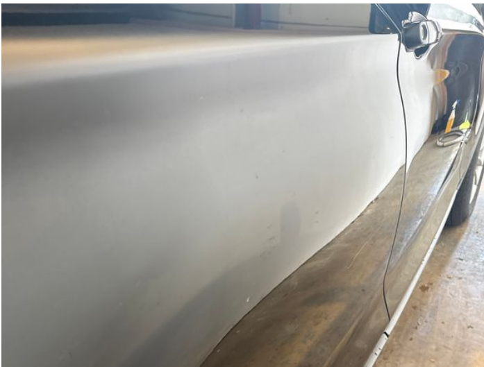
11: Door osr Dented With Paint Damage
