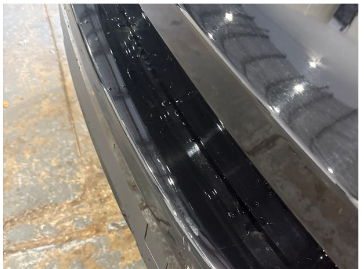
8: Bumper Rear Scratched 25 to 100mm Thru Paint
