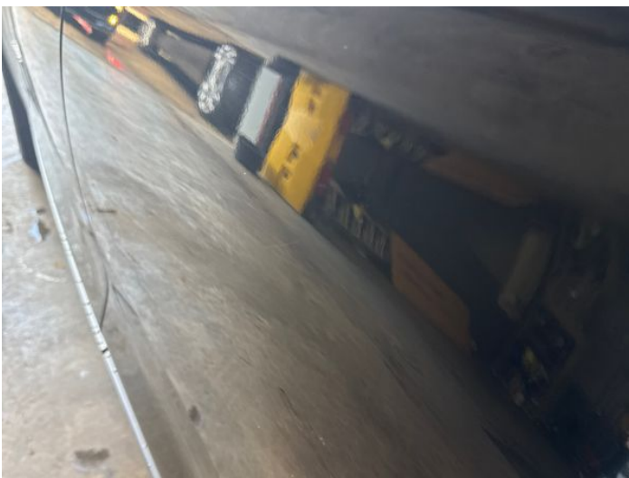
7: Door nsr Dented Between 10mm + 30mm
