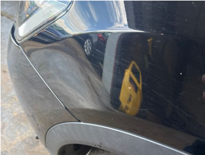
3: Wing nsf Scratched UpTo 25mm Thru Paint
