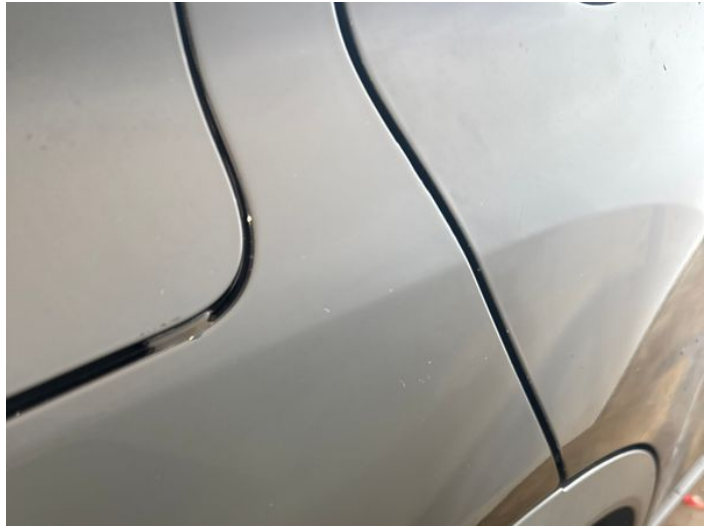
10: Qtr Panel osr Chipped 1 To 5
