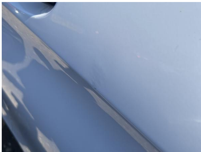
2: Door osf Poor Previous Repair Rippled UpTo 30%
