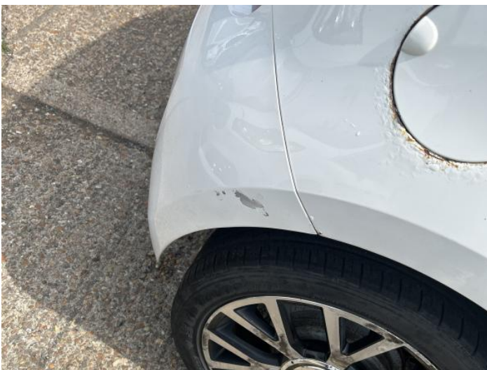
7: Bumper Rear Poor Previous Repair Paint Flake
