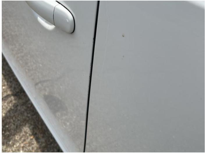
10: Door nsf Chipped Edge Chip
