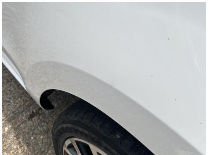
8: Qtr Panel nsr Dented 2 Or Less UpTo 10mm
