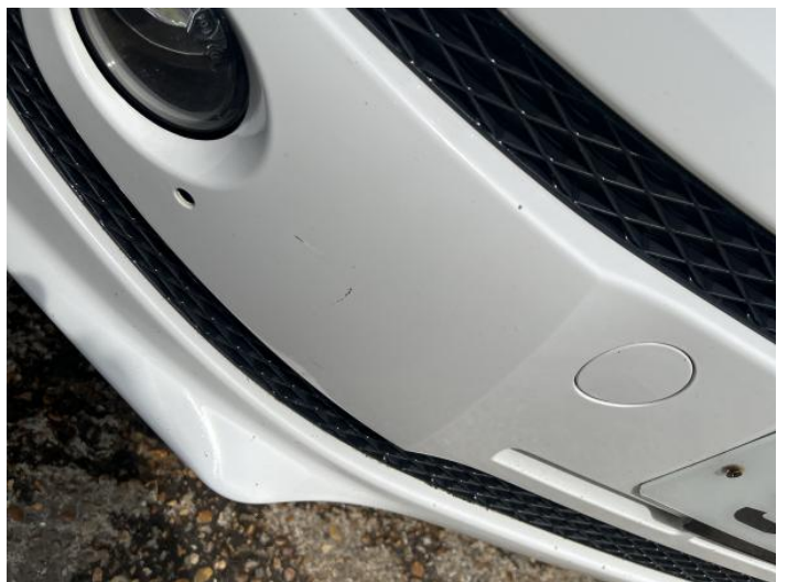
14: Bumper Front Scratched UpTo 25mm Thru Paint
