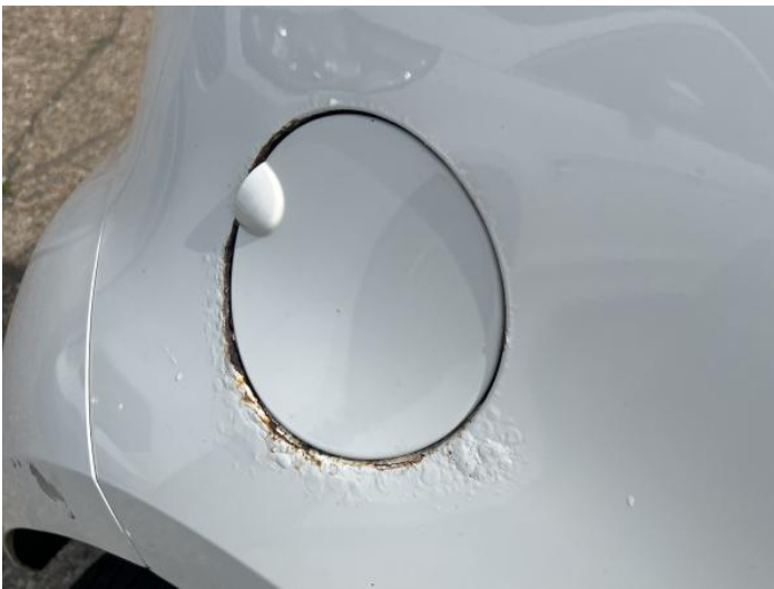
5: Qtr Panel osr Rusted Over 5mm
