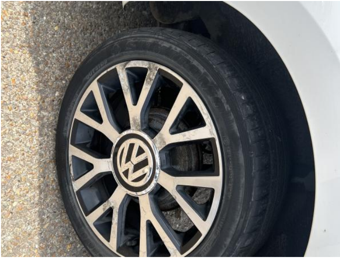
9: Wheel nsf Corroded Light
