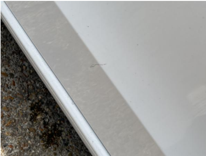
11: Door nsf Scratched UpTo 25mm Thru Paint
