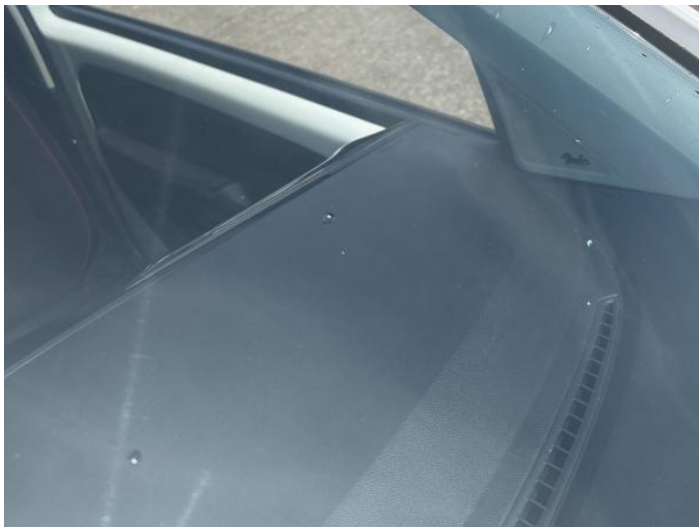
15: Screen Front Chipped UpTo 10mm
