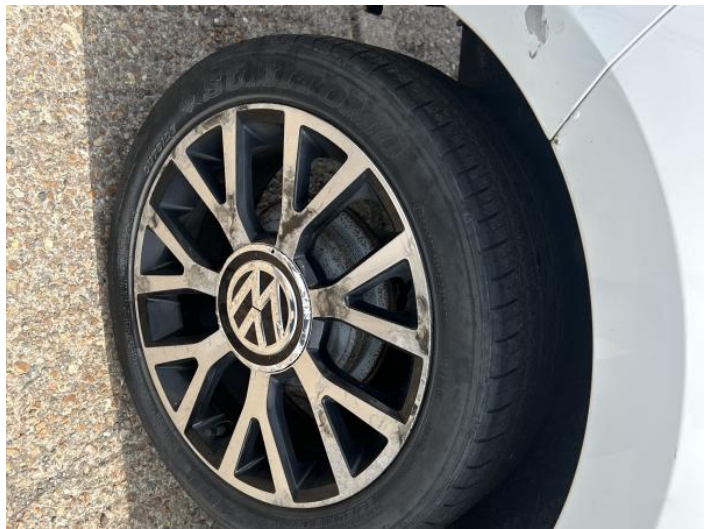
6: Wheel osr Corroded Light
