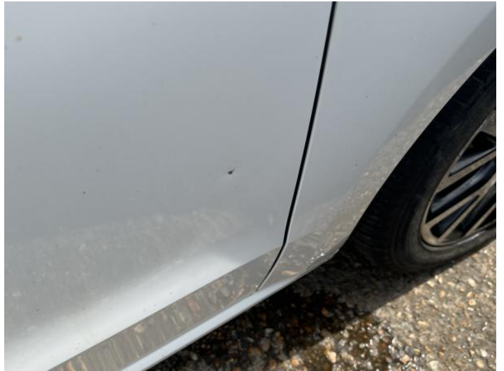
4: Door osf Dented With Paint Damage
