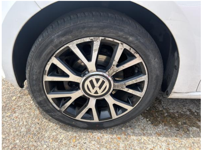
12: Wheel nsf Corroded Light
