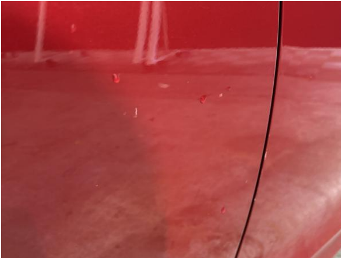
3: Door osr Chipped 1 To 5
