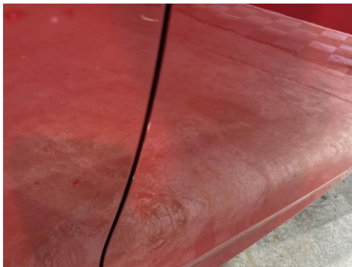
2: Door osf Chipped Edge Chip
