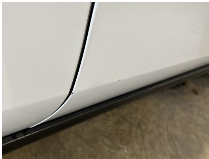
2: Door osf Chipped Edge Chip
