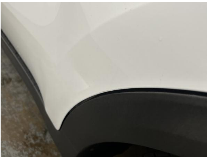
7: Door nsr Dented Over 30mm
