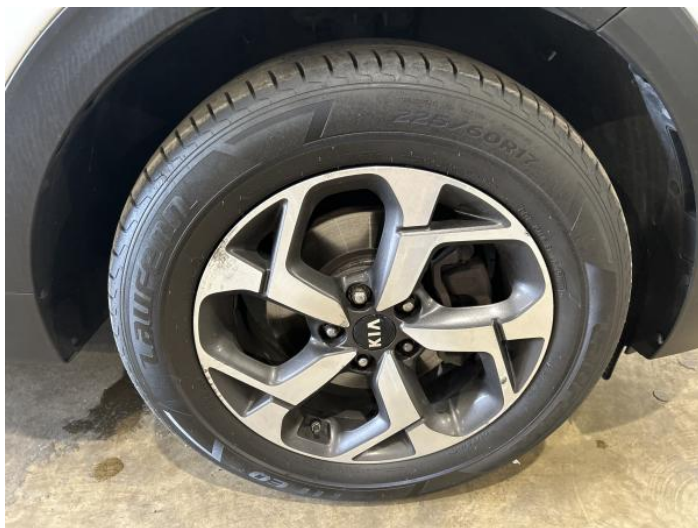
1: Wheel osf Corroded Light
