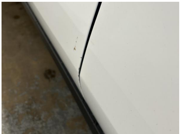
8: Door nsf Chipped Edge Chip
