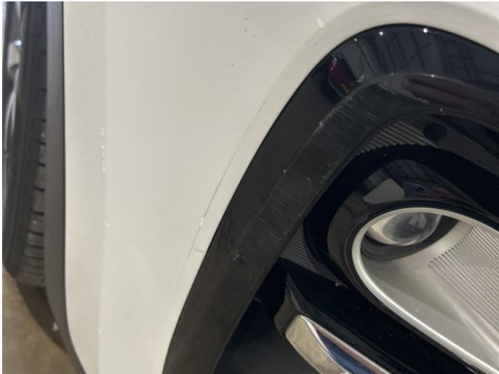
10: Bumper Front Scratched 25 to 100mm Thru Paint
