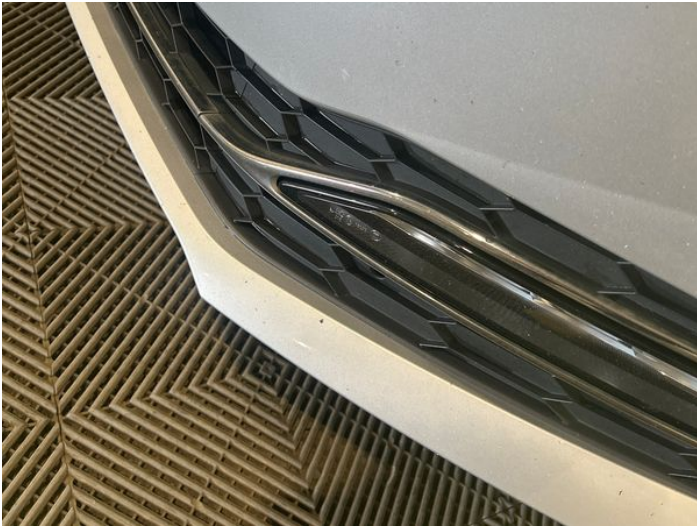
9: Bumper Front Chipped Multiple Chips
