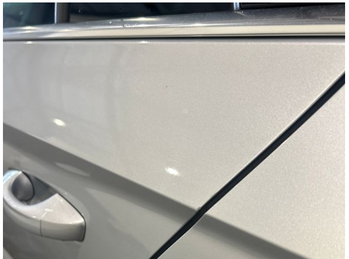
6: Door nsr Chipped Edge Chip
