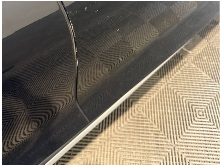
12: Door osf Scratched Over 25mm Thru Paint
