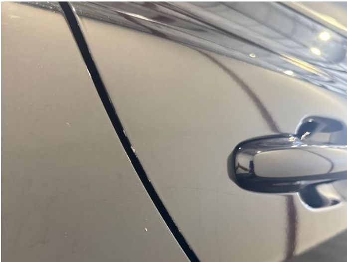
11: Door osr Chipped Edge Chip
