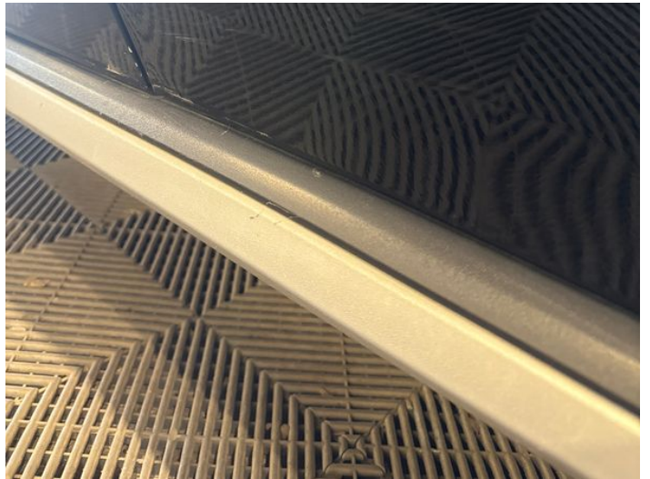
6: Door nsr Scratched Over 25mm Thru Paint
