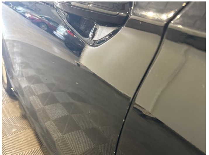
6: Door nsf Dented Over 30mm
