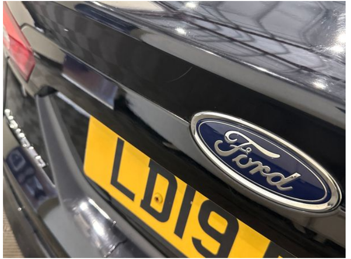
10: Boot Lid Scratched Over 25mm Thru Paint
