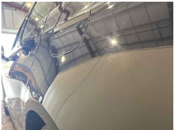
8: Qtr Panel nsr Poor Previous Repair Rippled UpTo 30%
