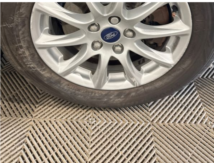
19: Wheel osf Scratched Over 50mm
