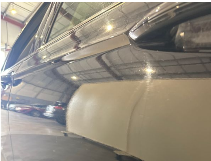
7: Door nsr Poor Previous Repair Rippled UpTo 30%
