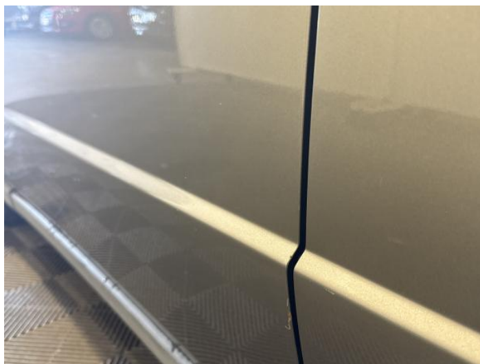
6: Door nsf Dented With Paint Damage
