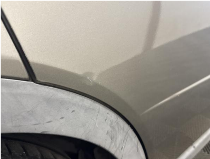
15: Door osr Dented Between 10mm + 30mm
