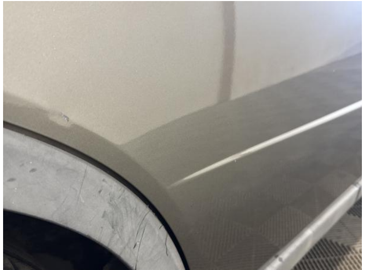
16: Door osr Scratched Over 25mm Thru Paint
