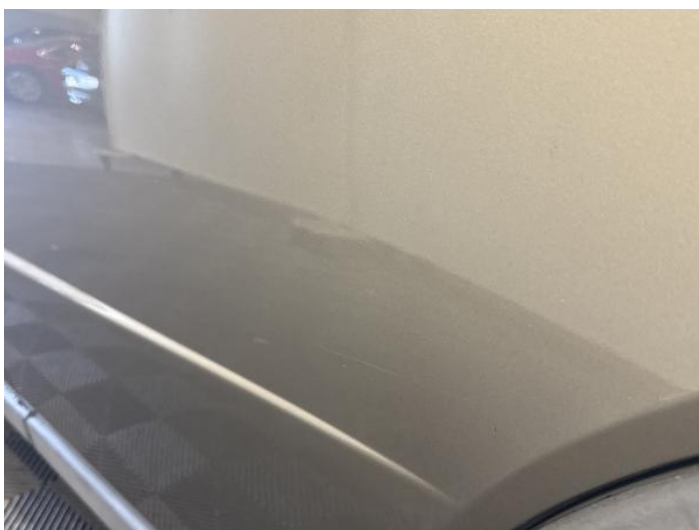
7: Door nsr Scratched Over 25mm Thru Paint
