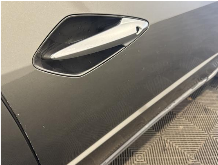
17: Door osf Dented With Paint Damage
