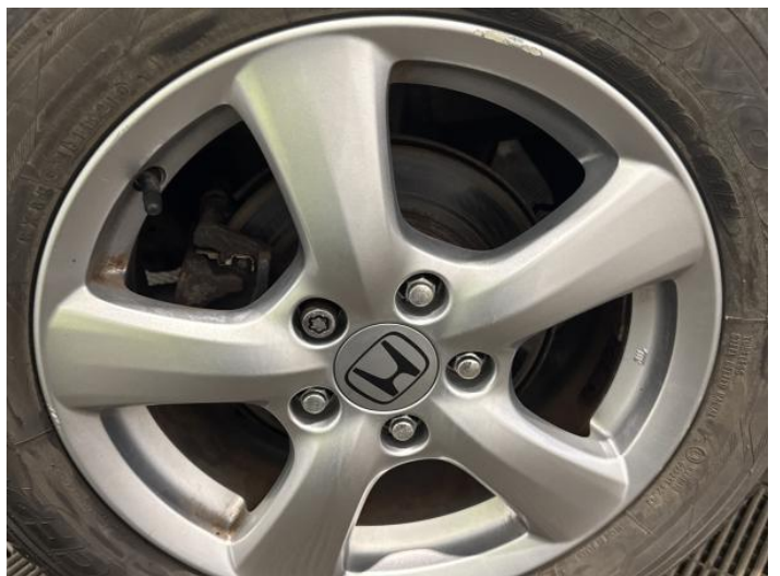
14: Wheel osr Scratched Over 50mm
