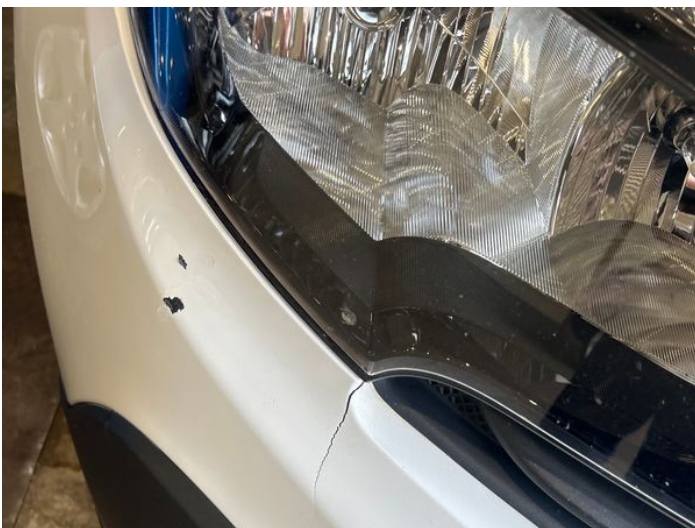
13: Bumper Front Cracked Over 25mm
