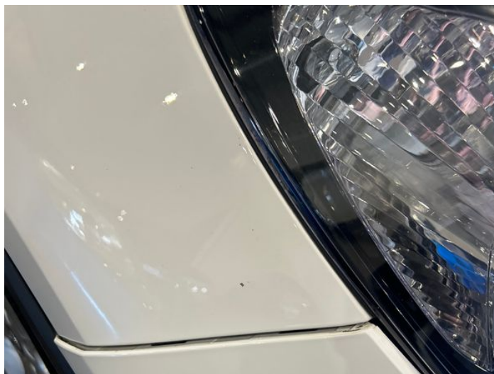
2: Wing osf Chipped 1 To 5
