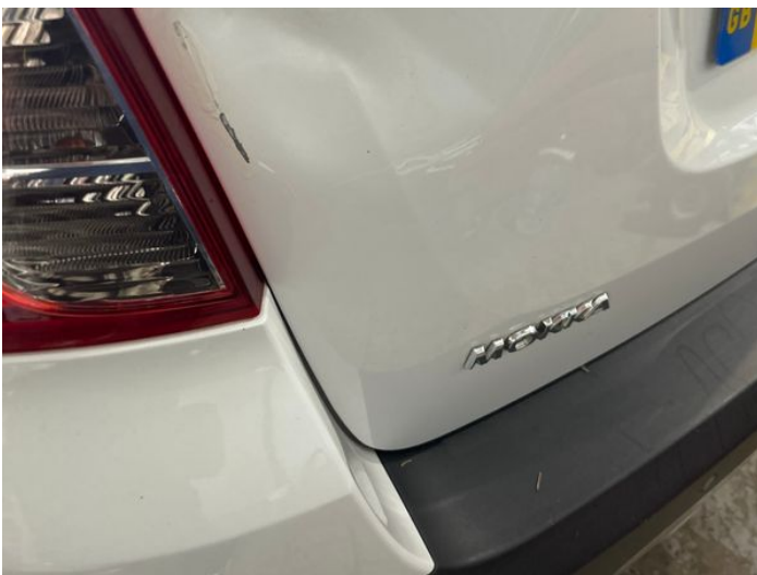
7: Tailgate Dented With Paint Damage
