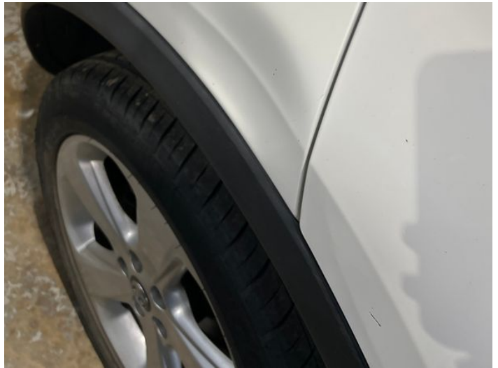
6: Qtr Panel osr Dented Over 30mm
