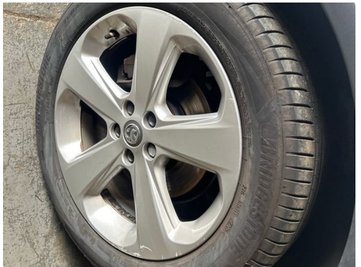
12: Wheel nsf Scratched Over 50mm
