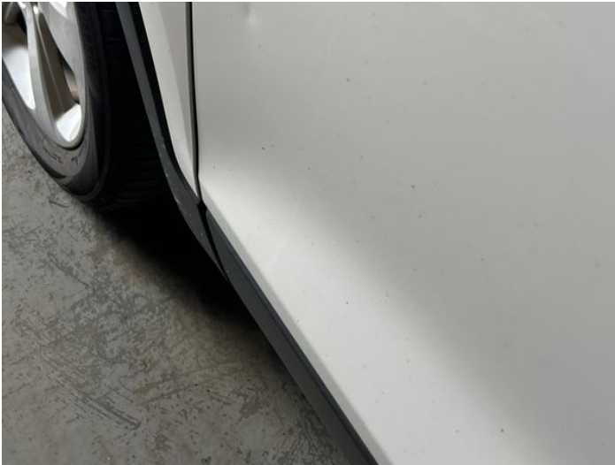
9: Door nsf Dented Between 10mm + 30mm
