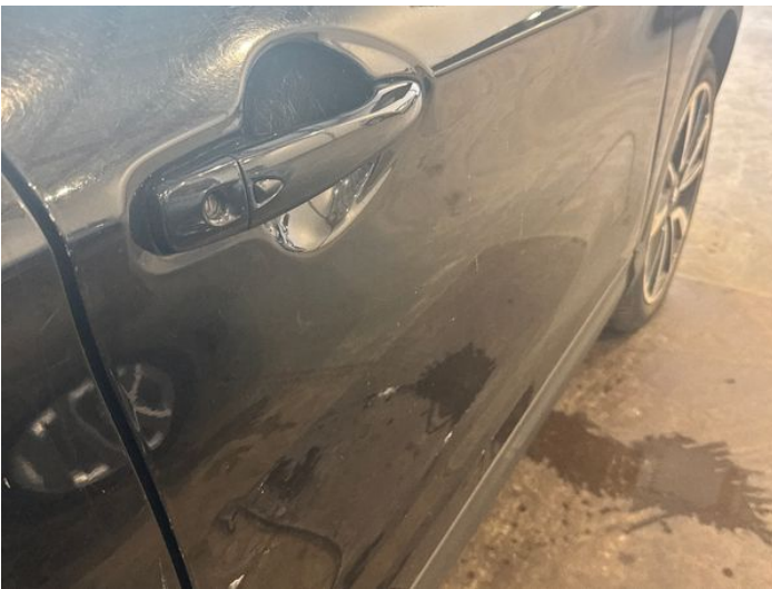
23: Door osf Dented With Paint Damage
