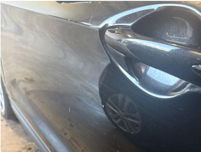
11: Door nsf Dented With Paint Damage
