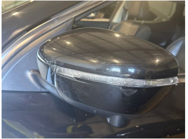
10: Door Mirror Assy nsf Broken Replace
