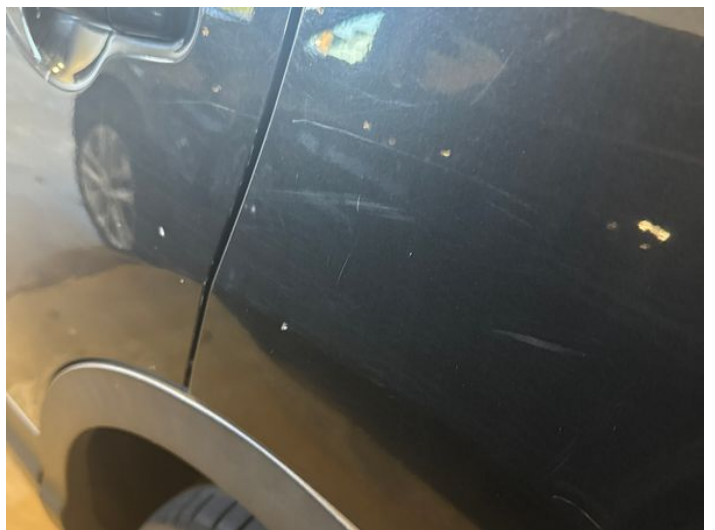
14: Qtr Panel nsr Dented Between 10mm + 30mm
