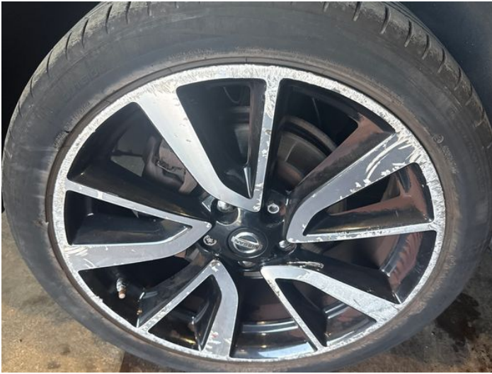
9: Wheel nsf Scratched Over 50mm
