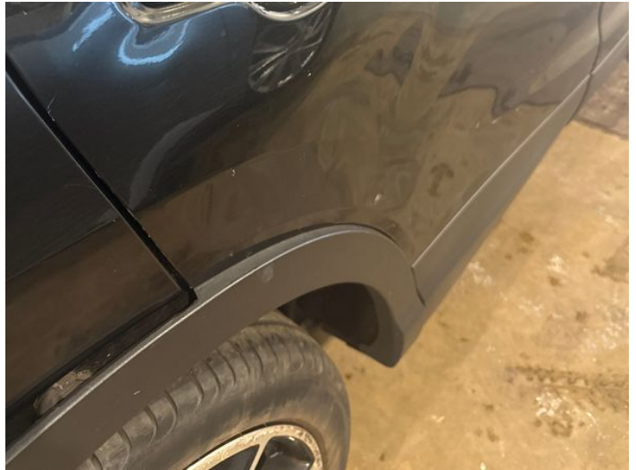
22: Door osr Dented With Paint Damage
