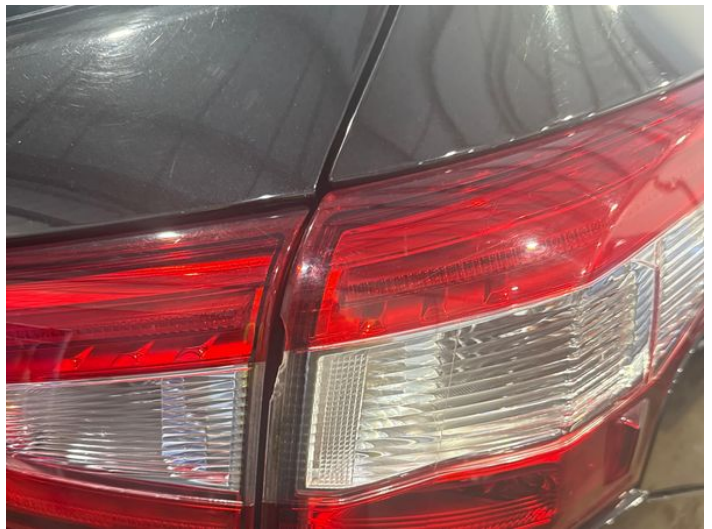
18: Lamp osr Broken Replace
