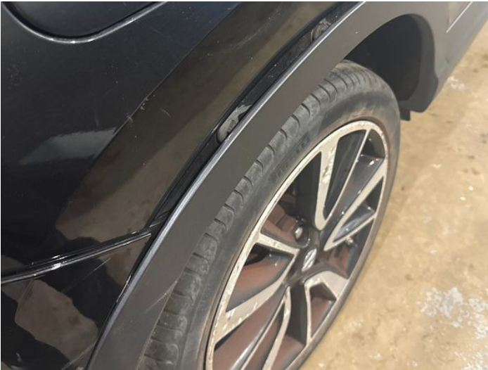
21: Qtr Panel Arch Extension os Broken Replace
