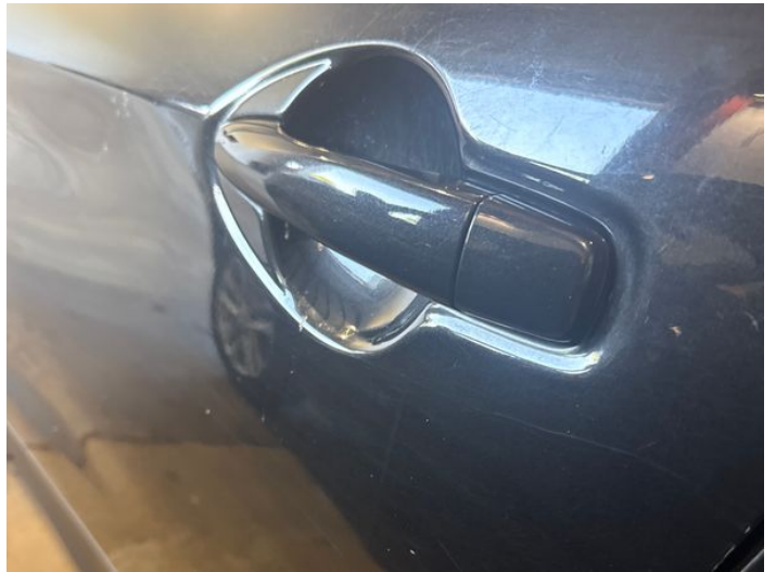
12: Door nsr Dented With Paint Damage
