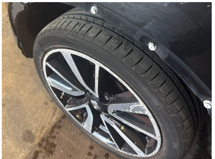
8: Wing Front Arch Extension ns Missing Replace
