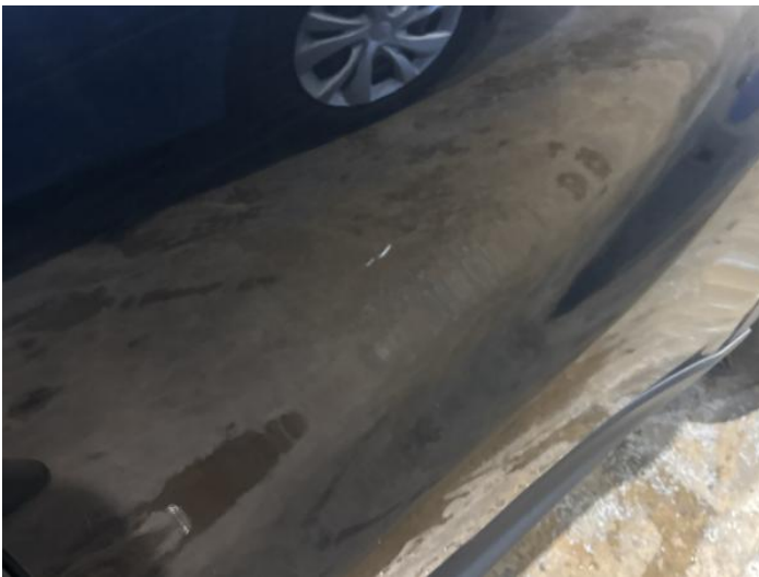
5: Door nsr Scratched UpTo 25mm Thru Paint
