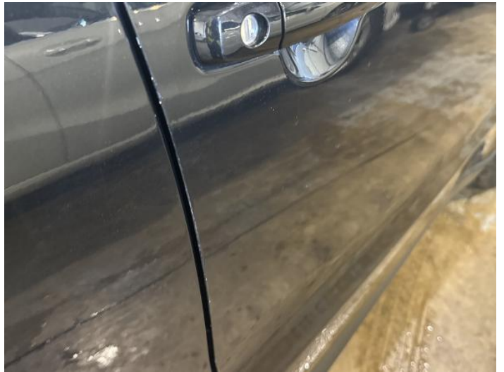
12: Door osf Chipped Edge Chip
