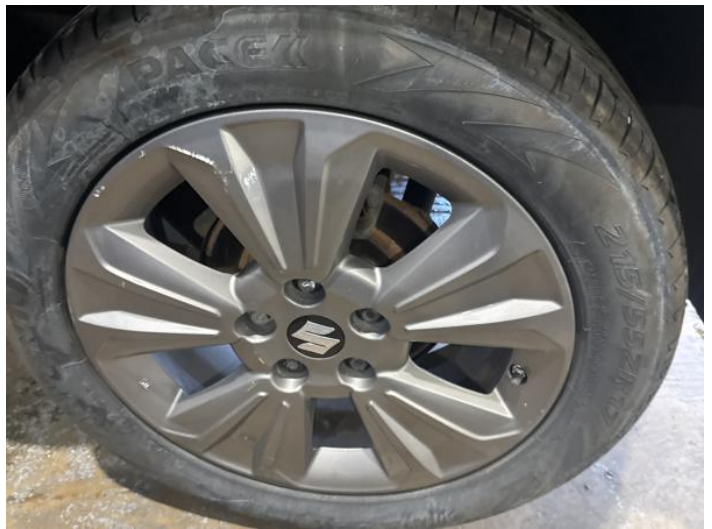
6: Wheel nsr Scratched Over 50mm
