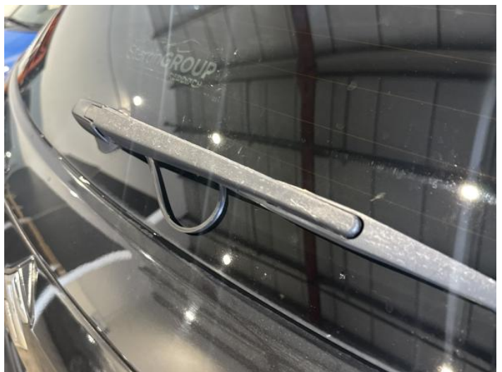
8: Wiper Rear Broken Replace
