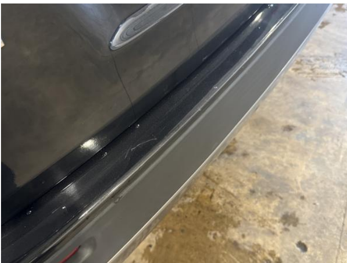
7: Bumper Rear Scratched 25 to 100mm Thru Paint
