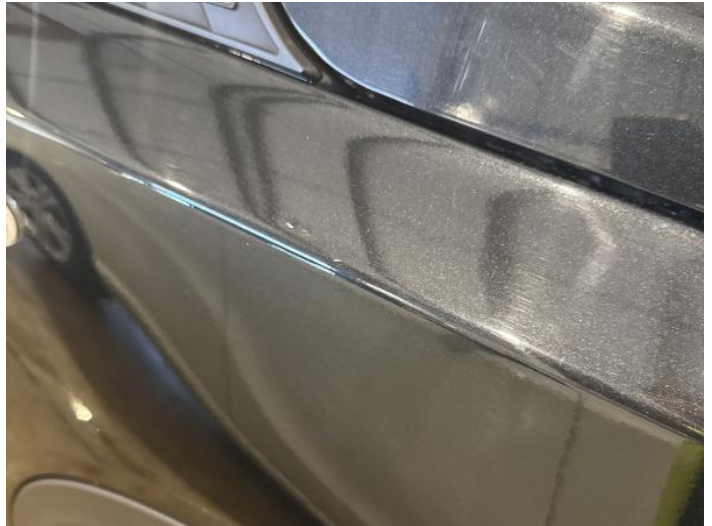
16: Wing osf Dented Between 10mm + 30mm
