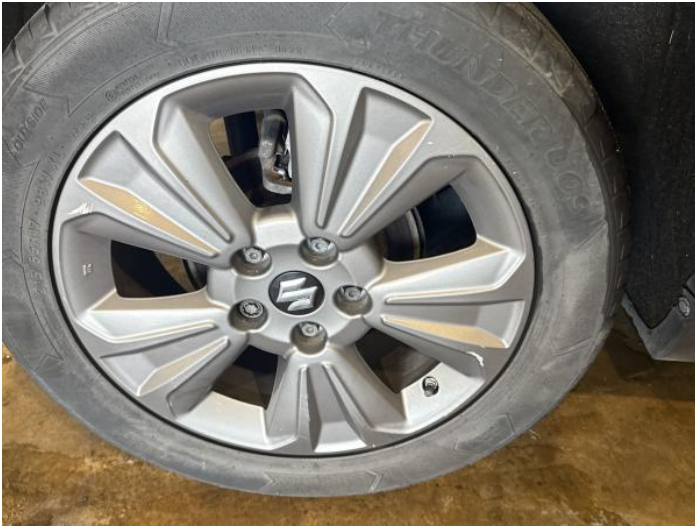
9: Wheel osr Scratched Over 50mm
