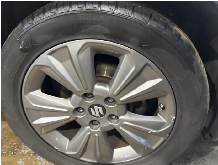
17: Wheel osf Scratched Over 50mm
