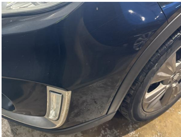
2: Bumper Front Scratched 25 to 100mm Thru Paint
