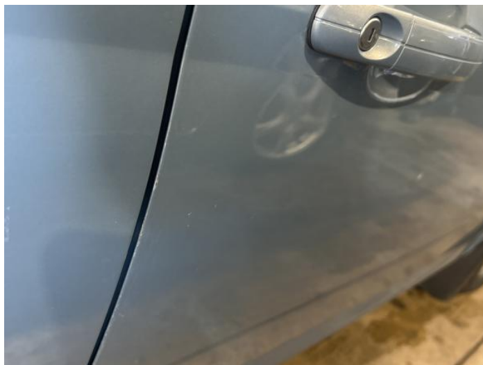
4: Door osf Chipped Edge Chip
