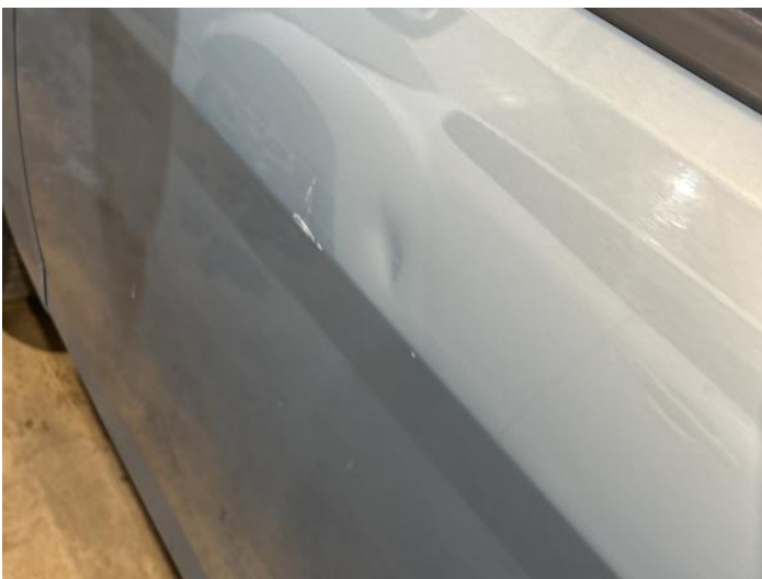
13: Door nsf Dented With Paint Damage
