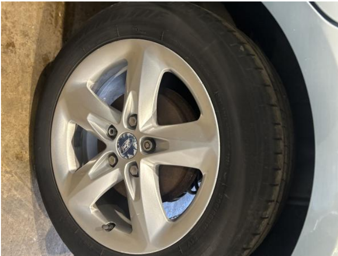
11: Wheel nsr Scratched Over 50mm
