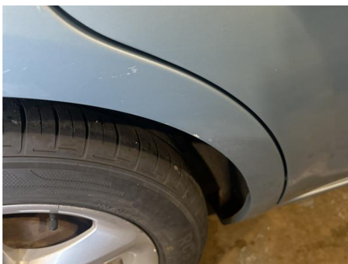
7: Qtr Panel osr Chipped 1 To 5
