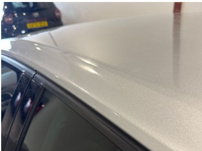
9: B Post ns Poor Previous Repair Poor Paint
