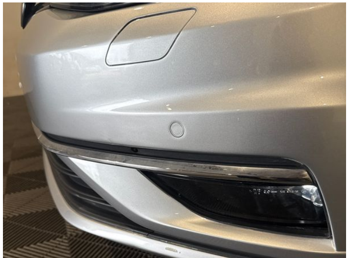
2: Bumper Front Poor Previous Repair Poor Paint
