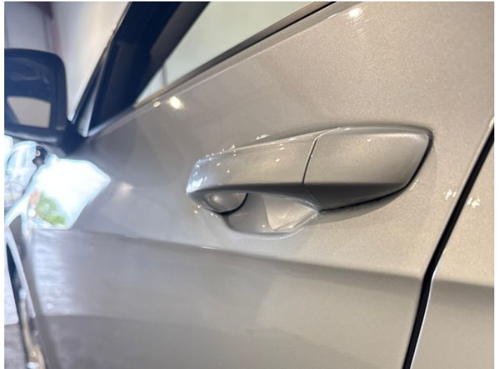
4: Door nsf Poor Previous Repair Poor Paint
