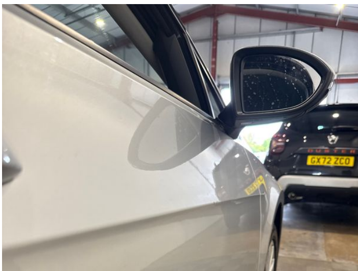
11: Door osf Dented Between 10mm + 30mm
