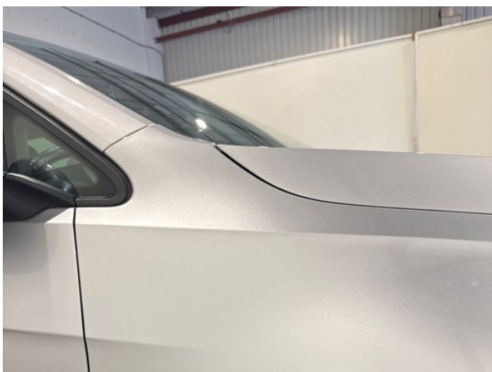
13: Wing osf Poor Previous Repair Poor Paint
