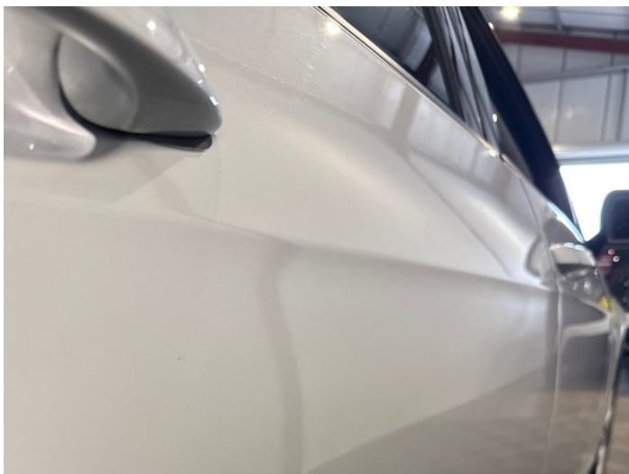
10: Door osr Poor Previous Repair Poor Paint
