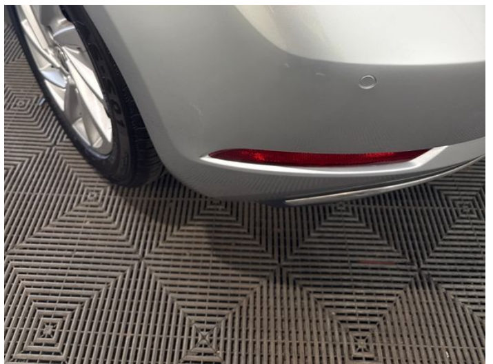
8: Bumper Rear Poor Previous Repair Poor Paint
