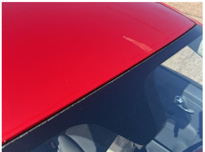
14: Roof Poor Previous Repair Paint Flake
