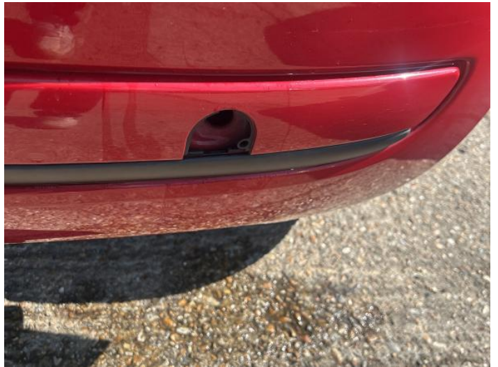
6: Rear TowEye Cvr Missing Replace
