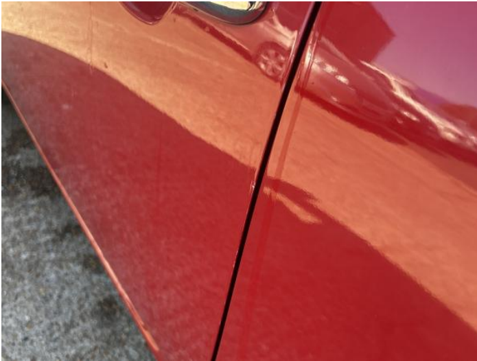
9: Door nsf Chipped Edge Chip
