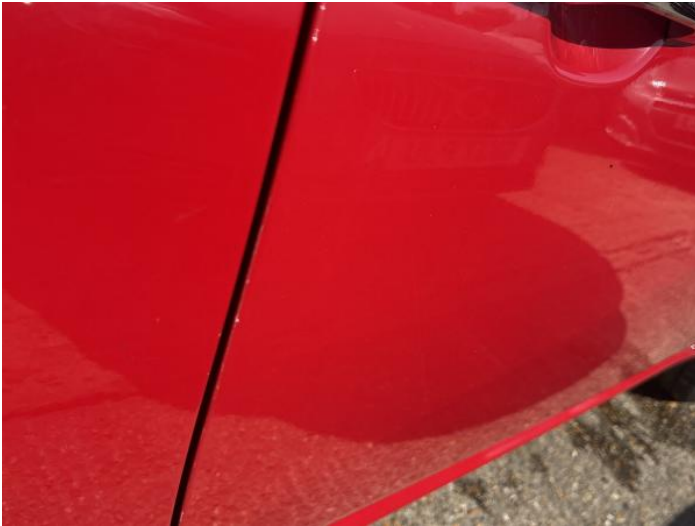
3: Door osf Chipped Edge Chip
