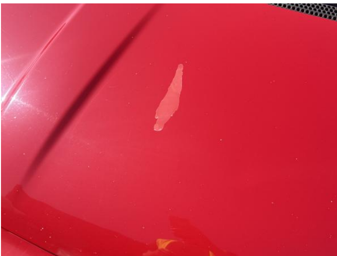
13: Bonnet Poor Previous Repair Paint Flake
