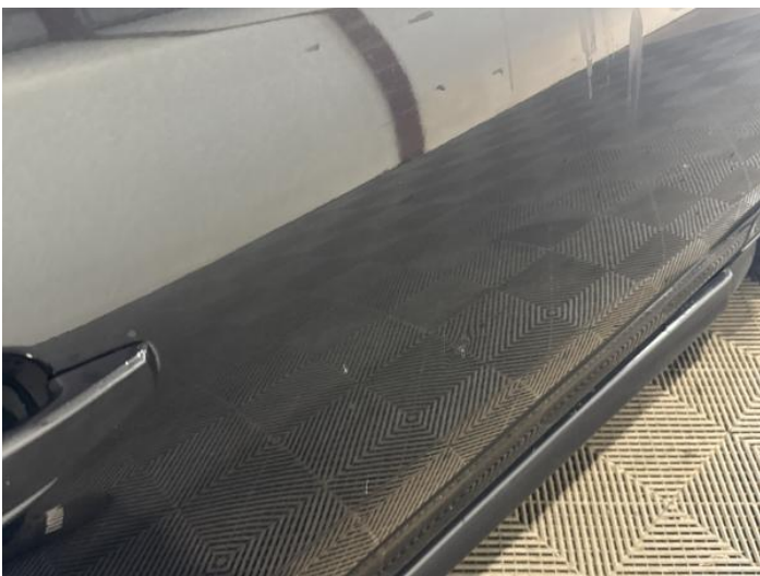
13: Door osf Dented With Paint Damage
