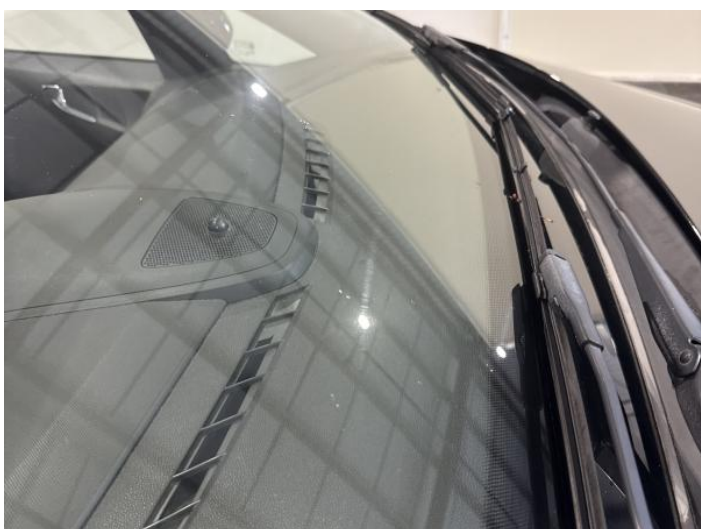
17: Screen Front Chipped UpTo 10mm
