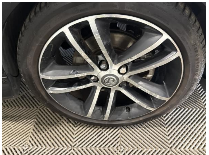
14: Wheel osf Scratched Over 50mm
