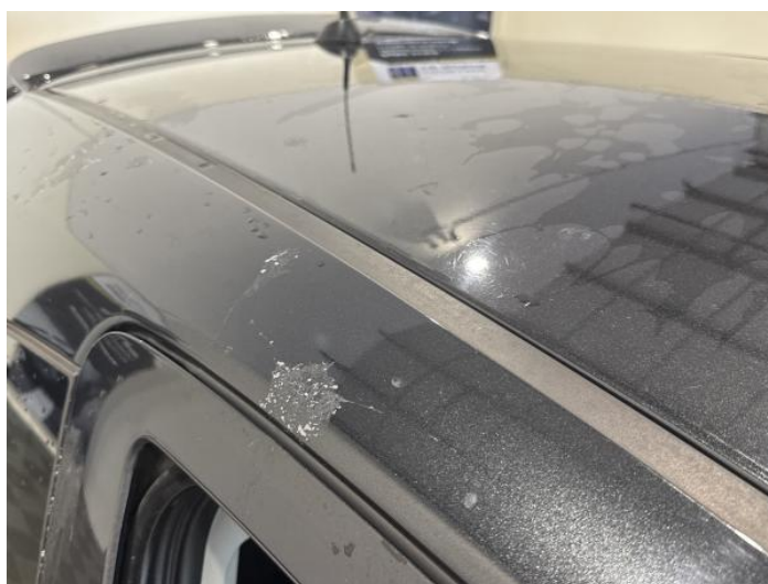
18: Roof Scratched Over 25mm Thru Paint
