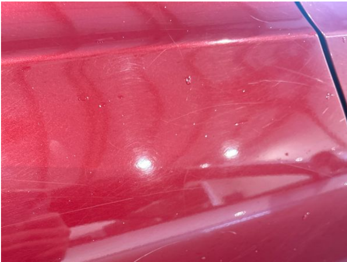
5: Door osr Scratched Over 25mm Thru Paint
