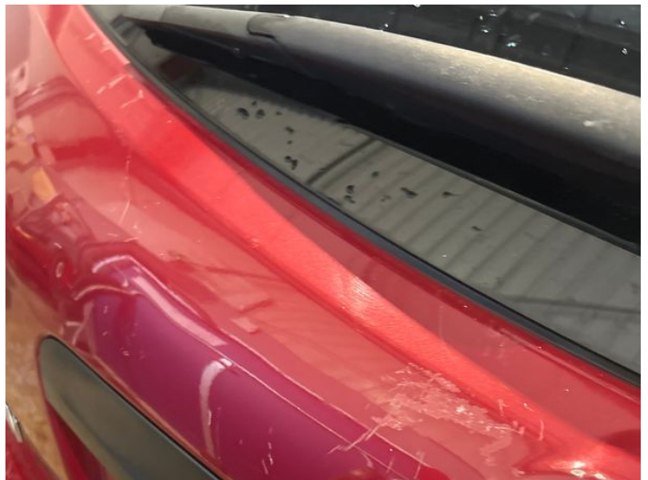
10: Tailgate Dented With Paint Damage
