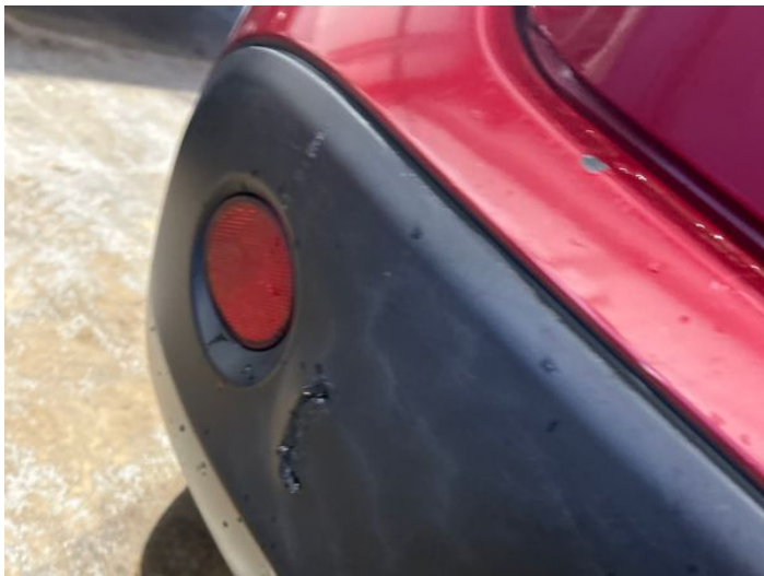
11: Bumper Rear Moulding Scuffed (Unpainted) UpTo 100mm
