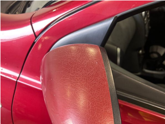
15: Door Mirror Assy nsf Scratched (Painted) Over 25mm Thru Paint
