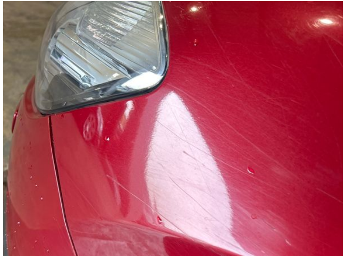
16: Wing nsf Scratched Over 25mm Thru Paint
