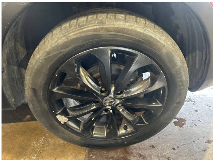
1: Wheel osf Scratched Over 50mm
