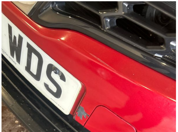
18: Bumper Front Poor Previous Repair Paint Flake
