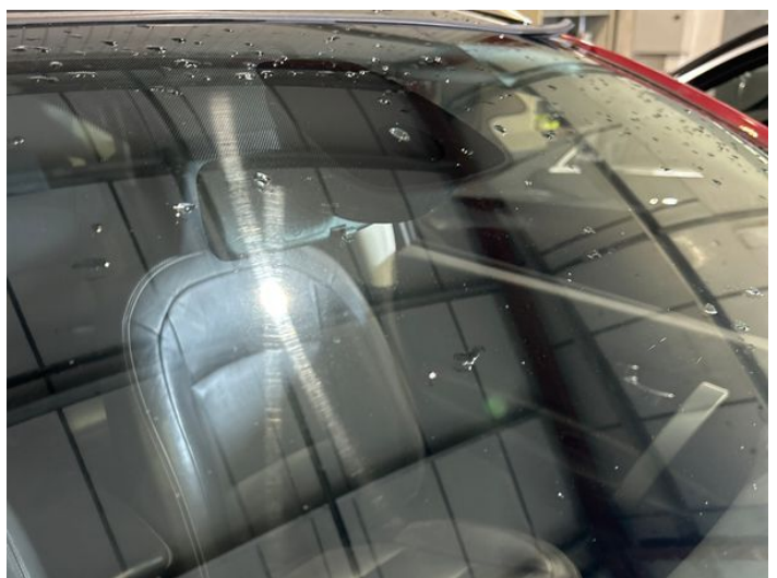
20: Screen Front Chipped UpTo 10mm
