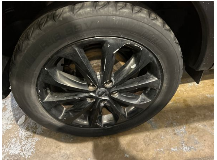
6: Wheel osr Scratched Over 50mm
