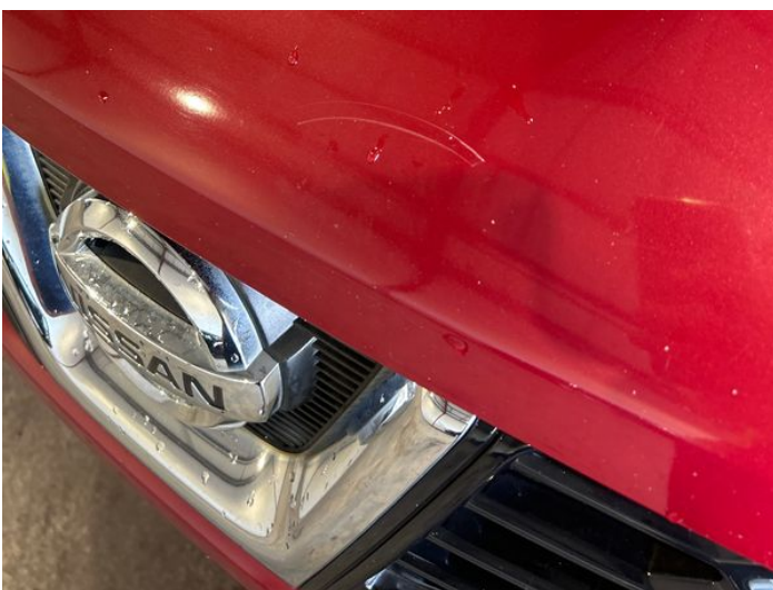
19: Bonnet Scratched Over 25mm Thru Paint
