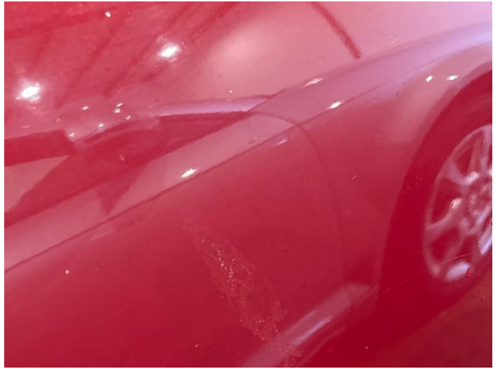
4: Door osf Poor Previous Repair Paint Flake
