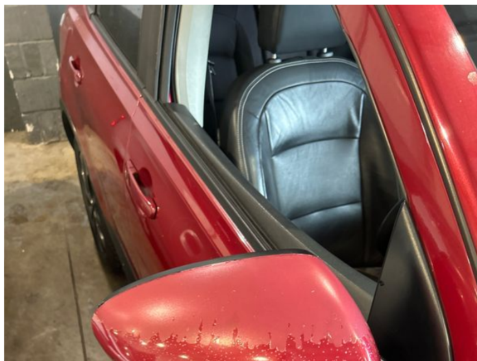
2: Door Mirror Assy osf Scratched (Painted) Over 25mm Thru Paint
