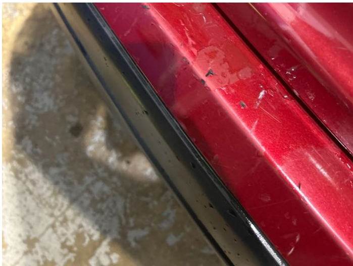
9: Bumper Rear Poor Previous Repair Paint Flake
