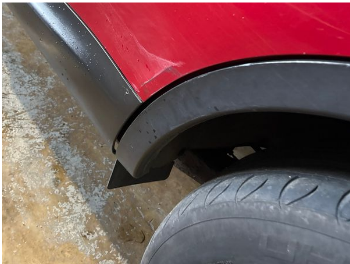
21: Door nsr Dented With Paint Damage
