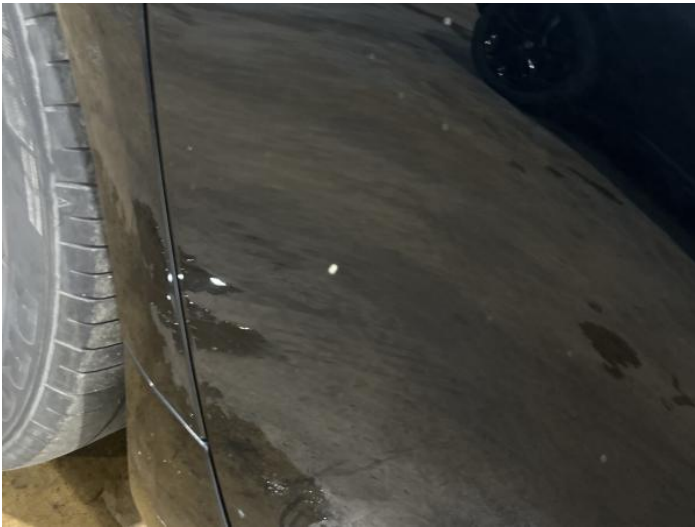
5: Door osr Chipped 1 To 5
