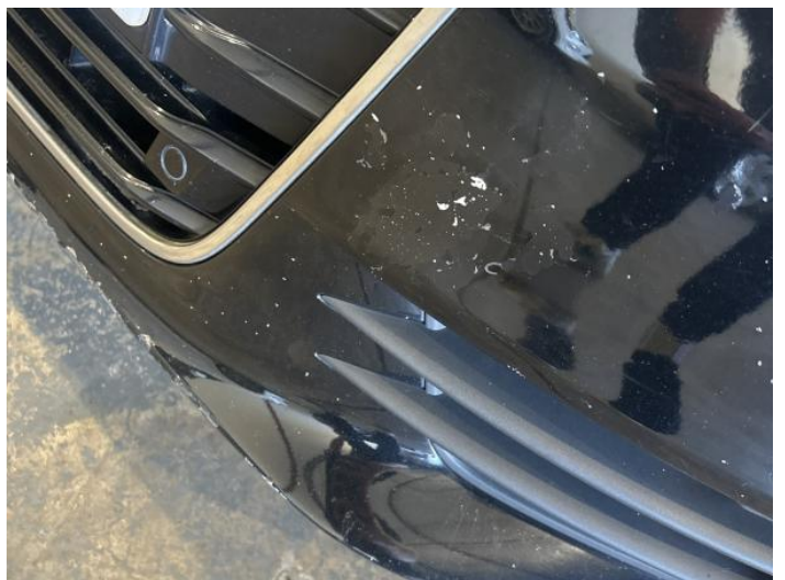
14: Bumper Front Poor Previous Repair Paint Flake
