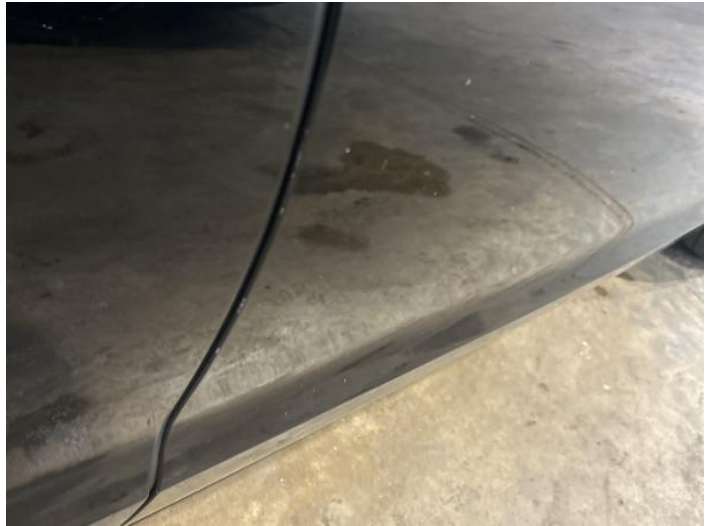
4: Door osf Chipped Edge Chip
