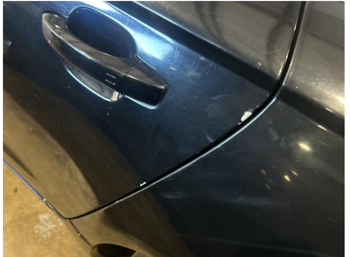
10: Door nsr Chipped Over 5mm
