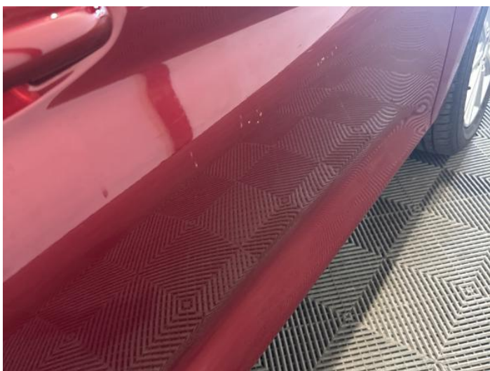
13: Door osf Dented With Paint Damage
