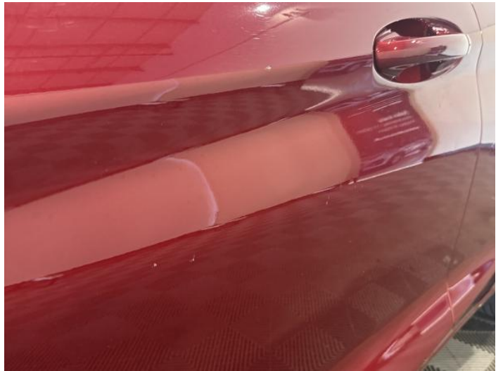
6: Door nsf Chipped Multiple Chips
