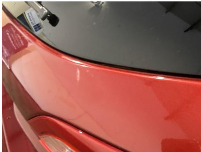
10: Tailgate Scratched Over 25mm Thru Paint
