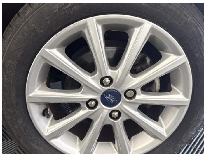
14: Wheel osf Scratched Over 50mm
