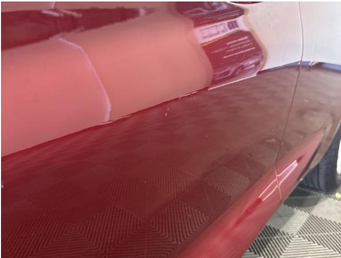
5: Door nsf Dented Over 30mm
