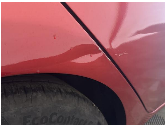
11: Qtr Panel osr Dented With Paint Damage
