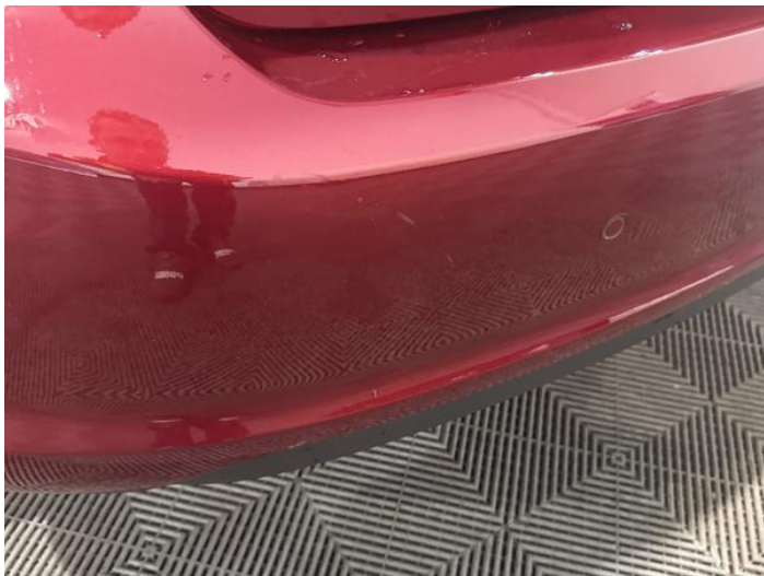
9: Bumper Rear Scratched 25 to 100mm Thru Paint
