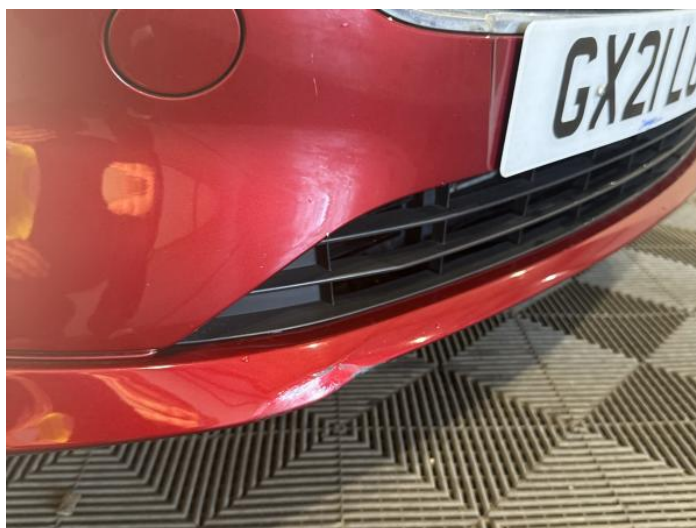
2: Bumper Front Dented With Paint Damage
