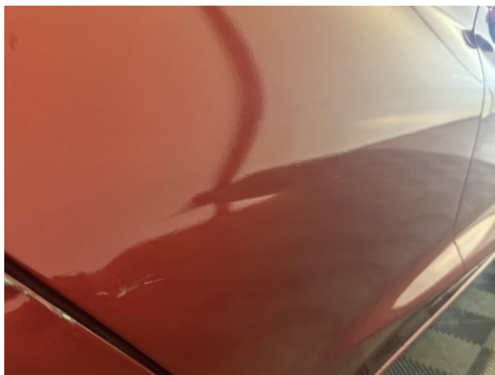
12: Door osr Dented With Paint Damage
