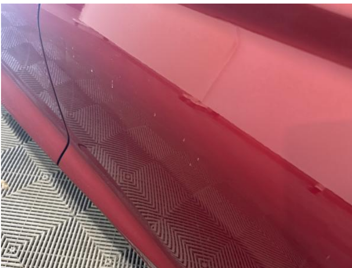
7: Door nsr Dented With Paint Damage
