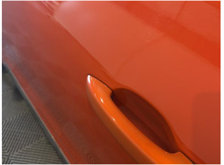
4: Door nsf Poor Previous Repair Poor Paint
