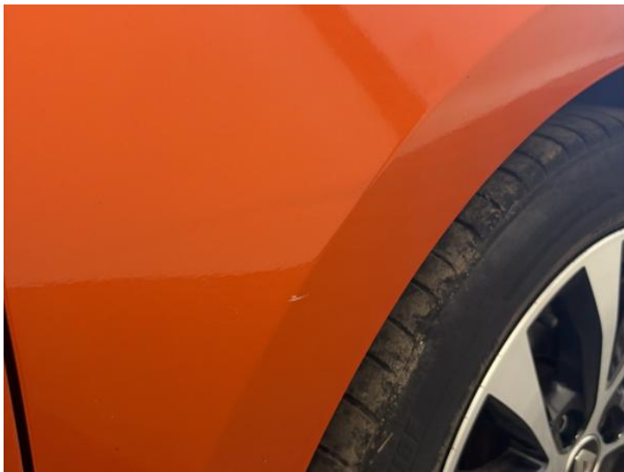
11: Wing osf Scratched UpTo 25mm Thru Paint
