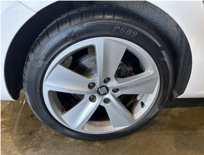
3: Wheel osr Corroded Light
