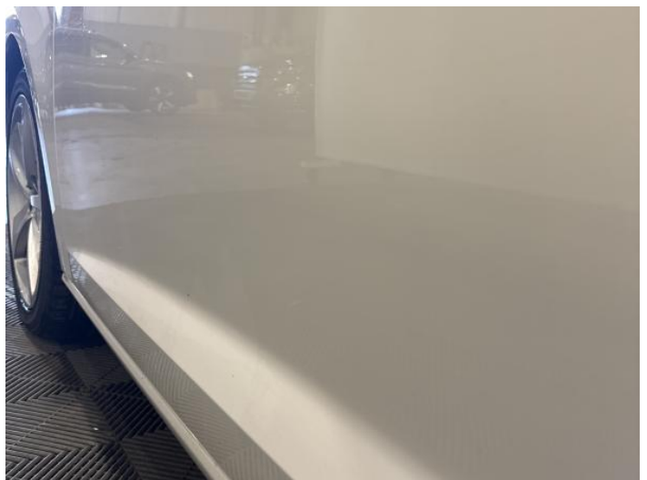
14: Door nsf Dented Over 30mm
