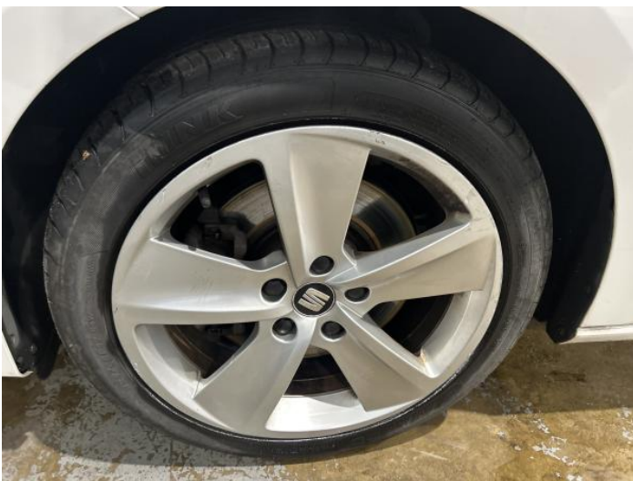
7: Wheel nsf Scratched Over 50mm
