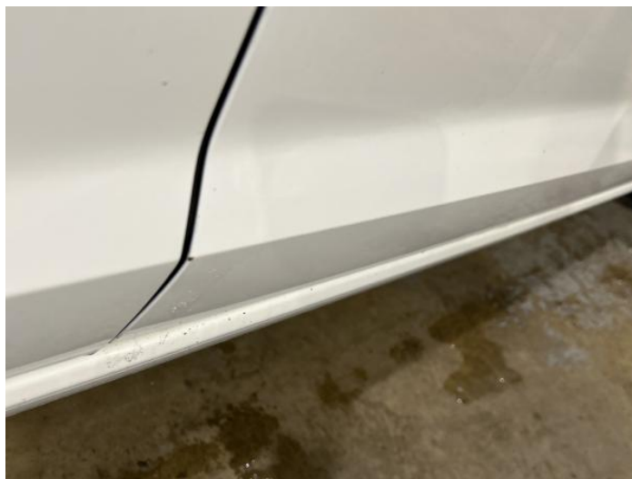
2: Door osf Chipped Edge Chip
