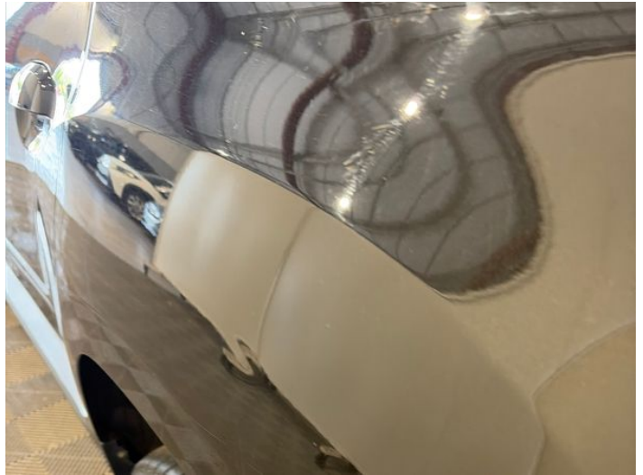
10: Qtr Panel nsr Dented Over 30mm
