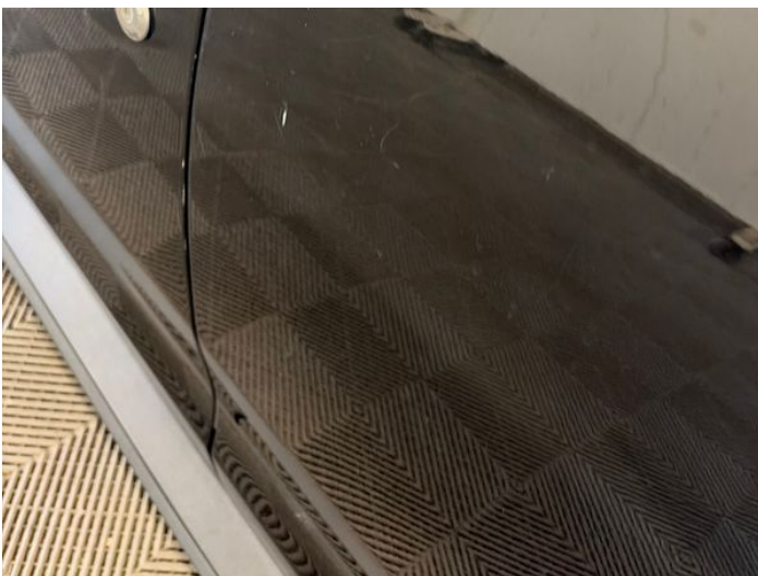
7: Door nsr Scratched Over 25mm Thru Paint
