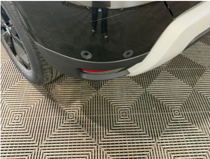
11: Bumper Rear Scratched 25 to 100mm Thru Paint
