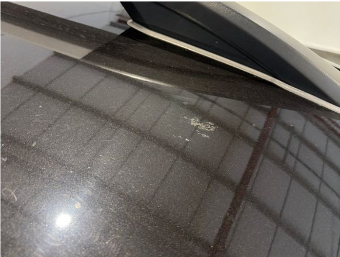
18: Roof Scratched Over 25mm Thru Paint
