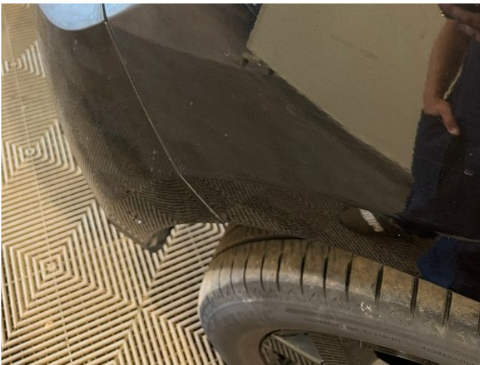
5: Wing nsf Scratched UpTo 25mm Thru Paint
