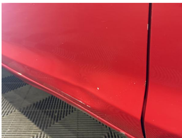
8: Door nsf Dented With Paint Damage
