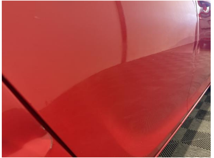
16: Door osf Dented With Paint Damage
