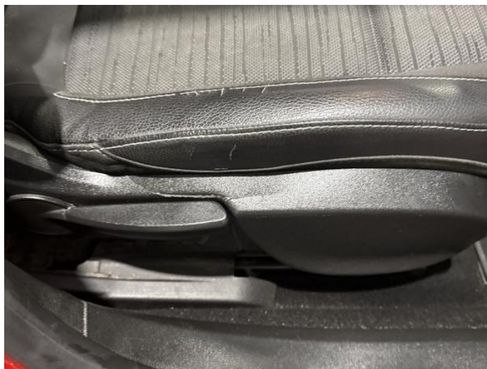
2: Fascia Trim Damaged Replace
