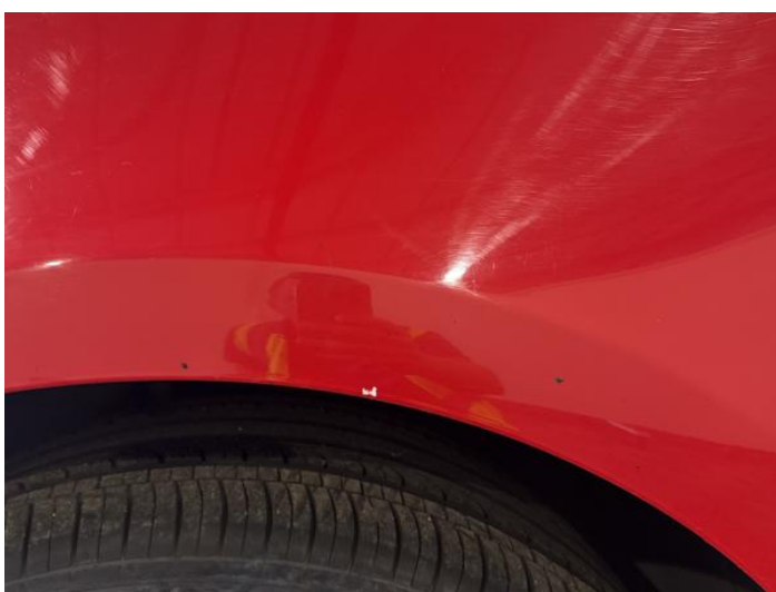
7: Wing nsf Chipped Over 5mm
