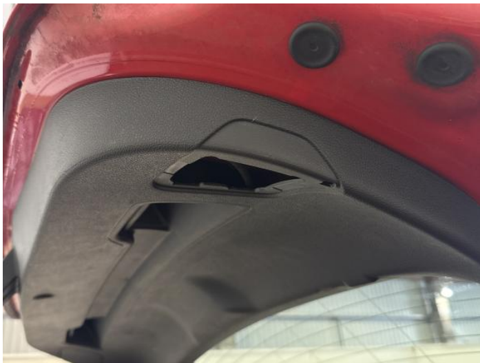
3: Fascia Trim Damaged Replace
