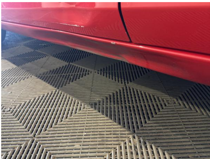
9: Sill ns Dented With Paint Damage
