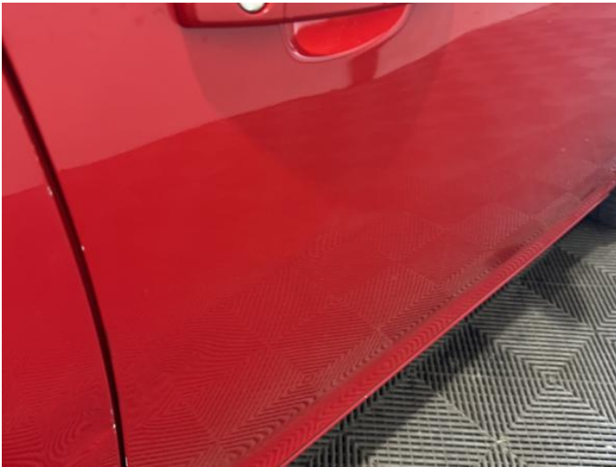
17: Door osf Dented With Paint Damage
