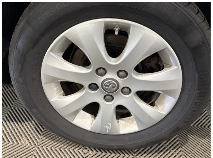
8: Wheel nsr Scratched Over 50mm
