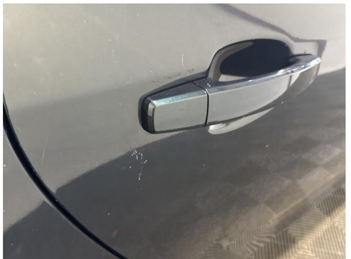
14: Door osr Scratched Over 25mm Thru Paint
