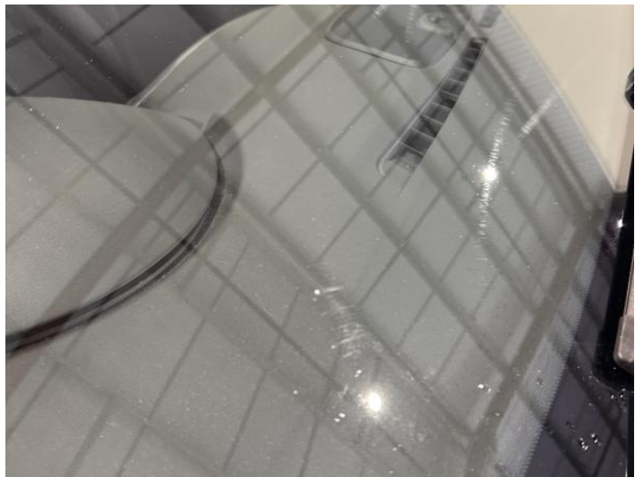
18: Screen Front Chipped UpTo 10mm
