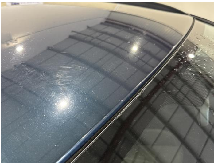
19: Roof Scratched Over 25mm Thru Paint
