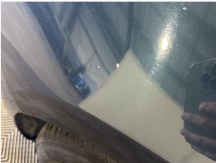
5: Wing nsf Scratched UpTo 25mm Thru Paint
