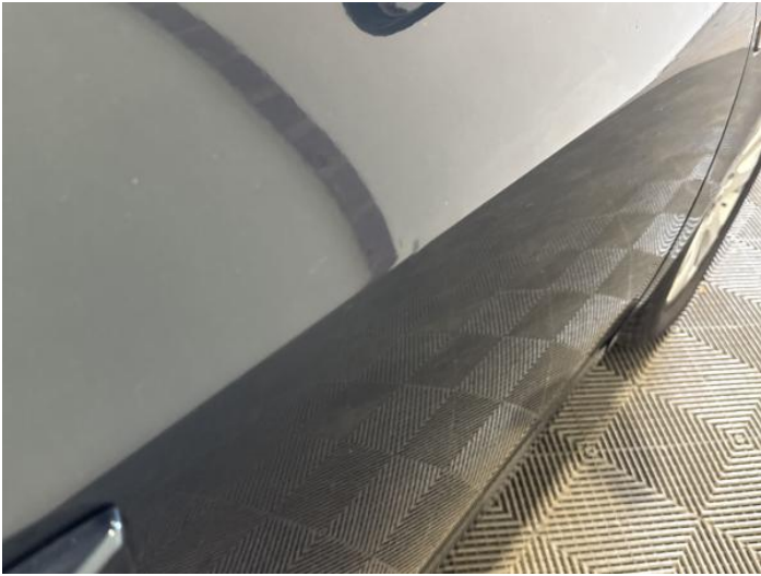
15: Door osf Dented Between 10mm + 30mm
