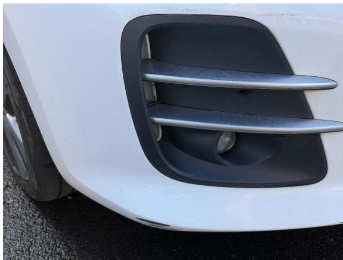
2: Bumper Front Scratched Over 100mm Thru Paint
