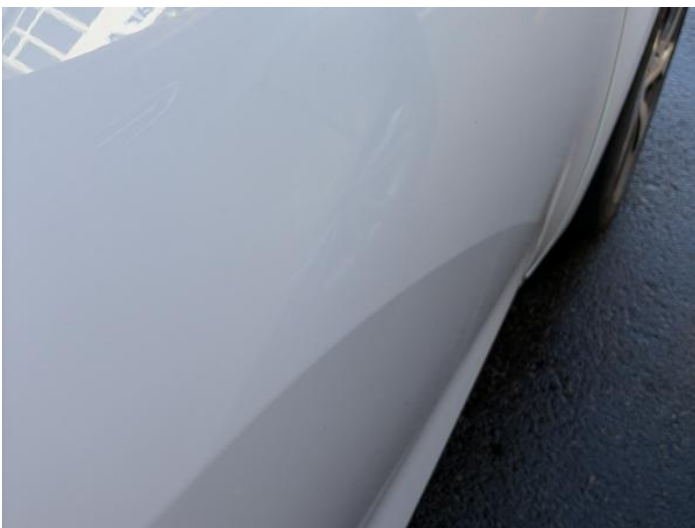
13: Door osf Dented Between 10mm + 30mm
