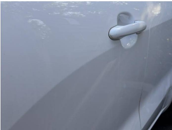
5: Door nsf Dented Between 10mm + 30mm
