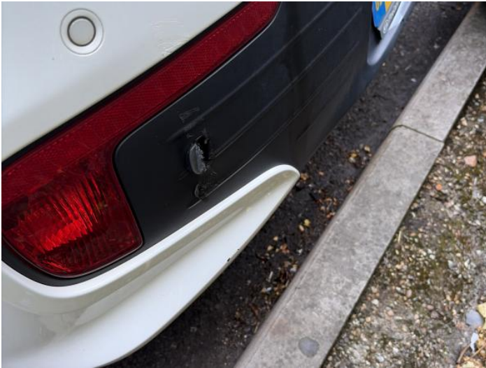
9: Bumper Rear Moulding Broken Replace
