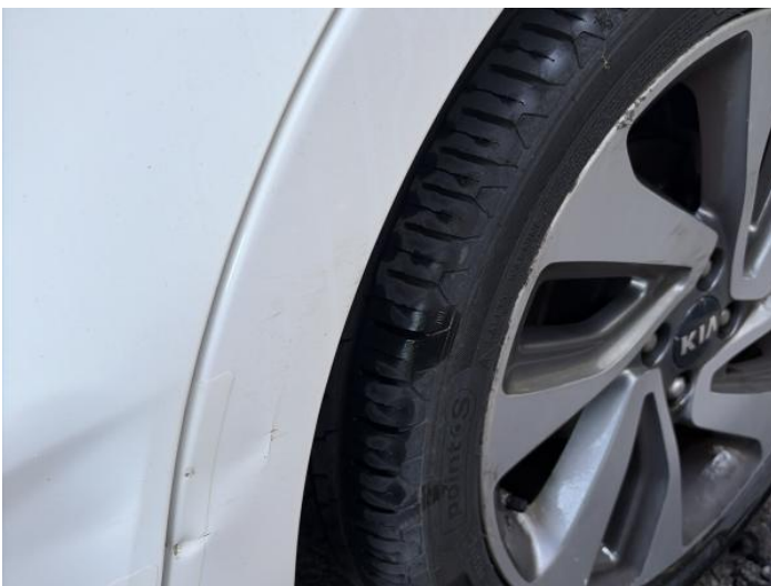
7: Qtr Panel nsr Dented With Paint Damage
