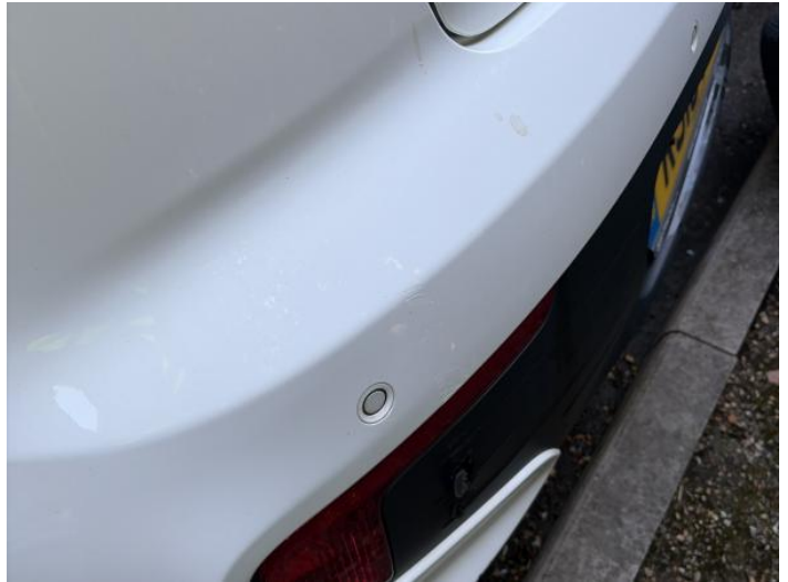
10: Bumper Rear Scratched 25 to 100mm Thru Paint
