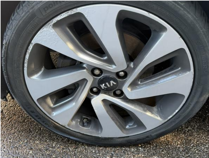
3: Wheel nsf Scratched Over 50mm
