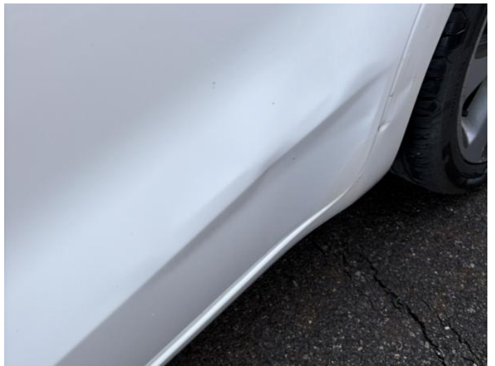
6: Door nsr Dented Over 30mm
