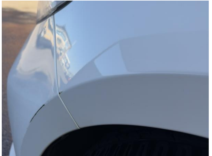
4: Wing nsf Scratched UpTo 25mm Thru Paint
