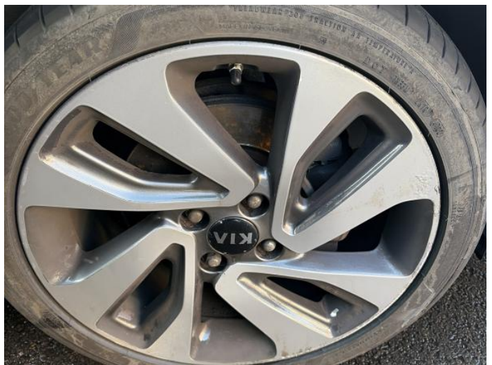
14: Wheel osf Scratched Over 50mm
