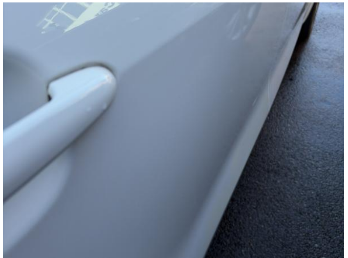
12: Door osr Dented Between 10mm + 30mm
