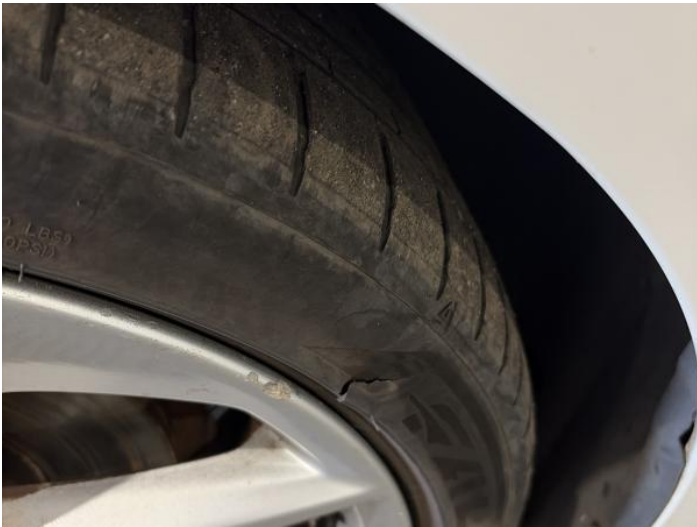
17: Tyre nsf Damaged Replace
