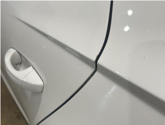
9: Door nsr Chipped Edge Chip
