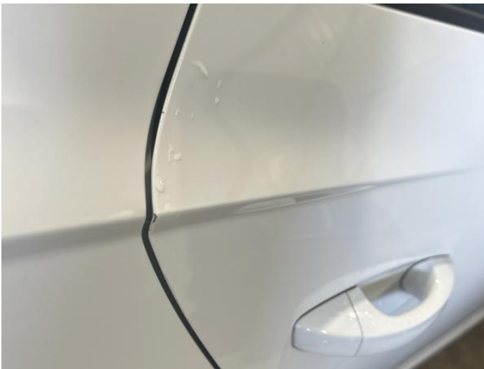
5: Door osr Chipped Edge Chip
