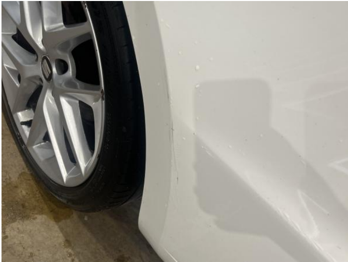
16: Bumper Rear Scratched 25 to 100mm Thru Paint
