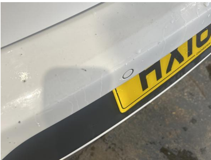
7: Bumper Rear Chipped Multiple Chips
