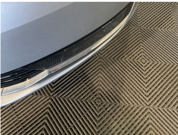
13: Bumper Front Chipped Multiple Chips
