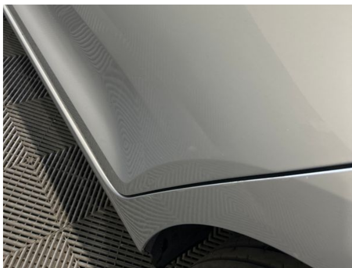
8: Door nsr Dented Over 30mm
