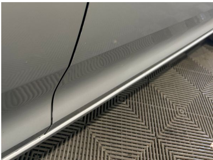
3: Door osf Chipped Edge Chip
