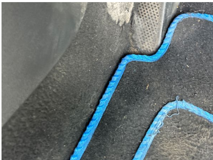
1: Carpets Front Scuffed Over 25mm
