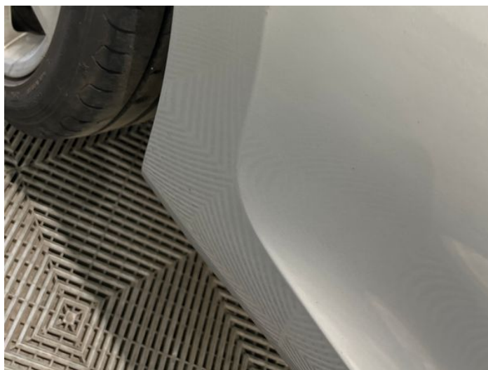
6: Bumper Rear Scratched Up To 25mm Thru Paint
