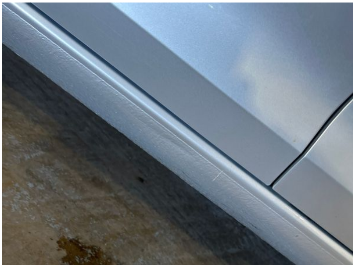
15: Sill ns Dented Over 30mm
