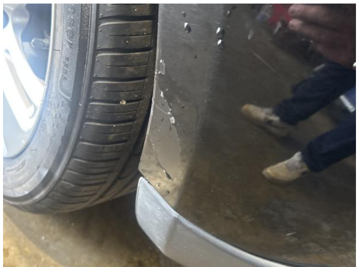
8: Bumper Rear Poor Previous Repair Paint Flake
