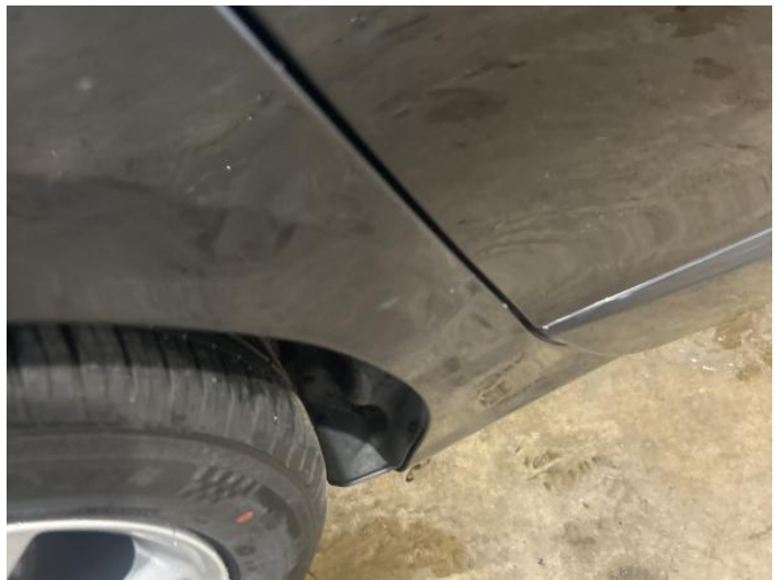
6: Qtr Panel osr Dented Over 30mm
