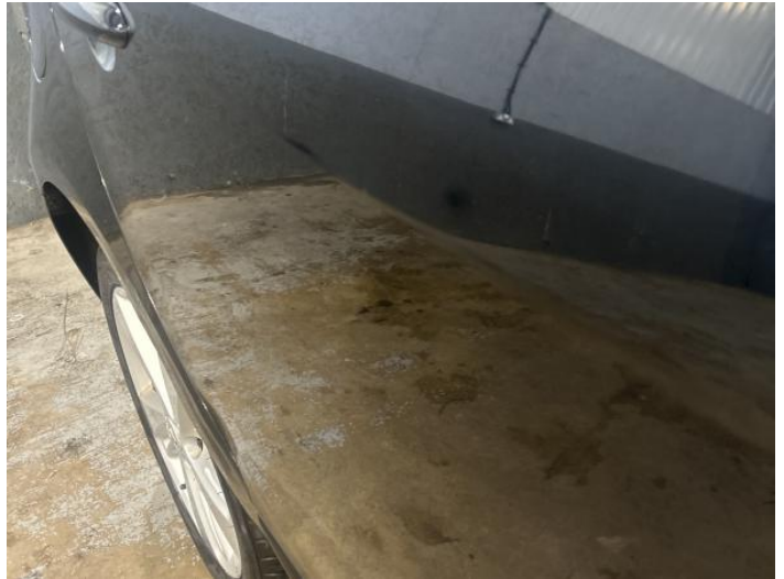
4: Door osr Dented 2 Or Less UpTo 10mm
