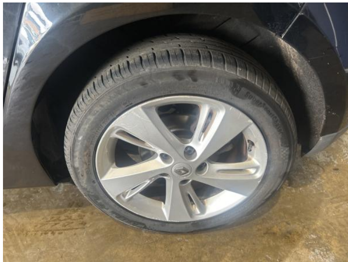
10: Wheel nsr Scratched Over 50mm
