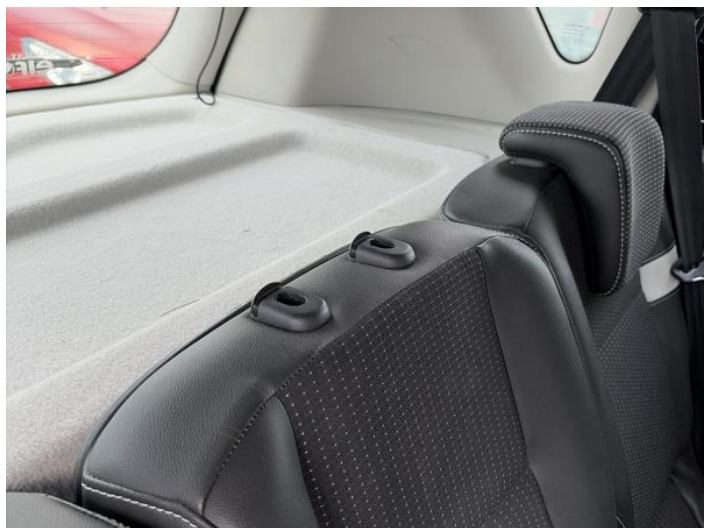
20: Headrest Assy Rear Seat Centr Missing Replace
