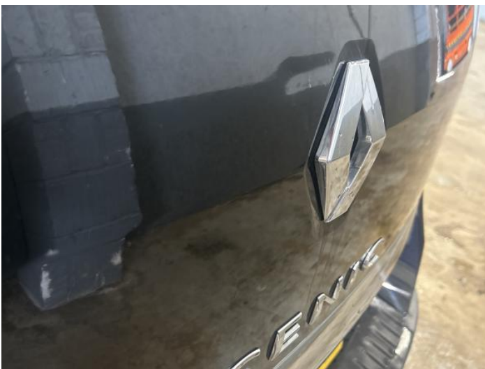
7: Tailgate Dented With Paint Damage
