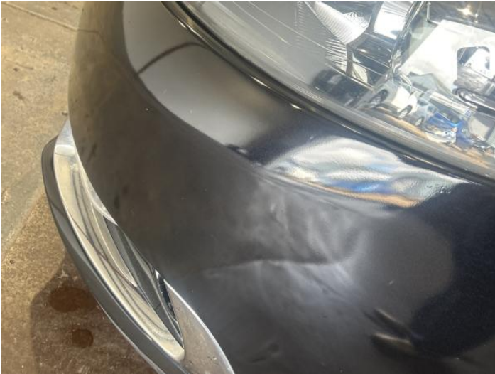
15: Bumper Front Poor Previous Repair Poor Paint
