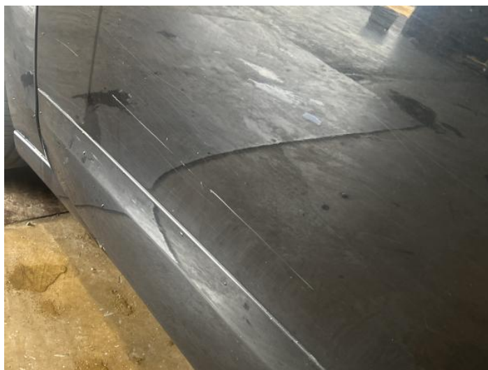
12: Door nsf Scratched Over 25mm Thru Paint
