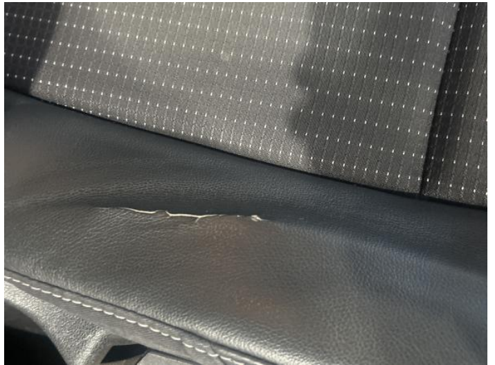
18: Seat Base Cover osf Torn Over 3mm
