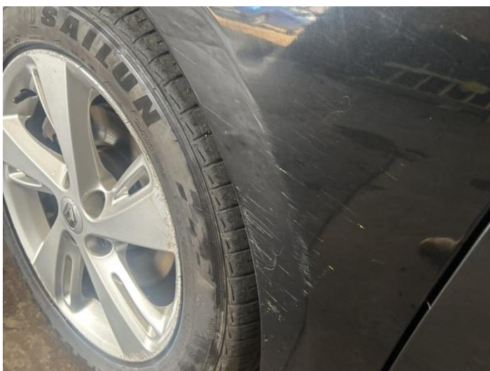
13: Wing nsf Scratched Over 25mm Thru Paint
