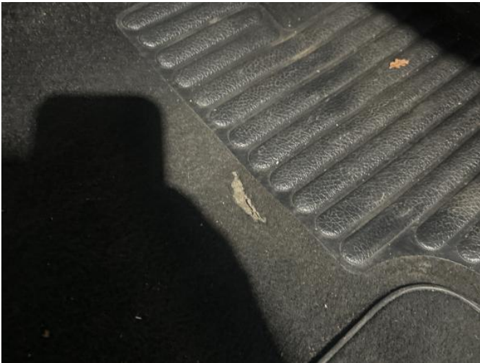
17: Carpets Front Holed Over 3mm
