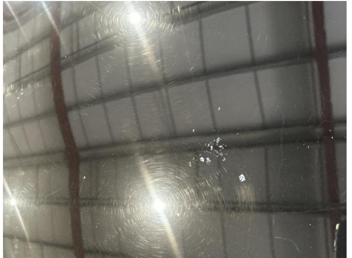
16: Bonnet Chipped Multiple Chips
