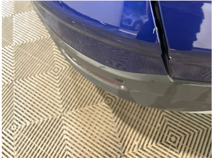
4: Bumper Rear Chipped 1 To 5
