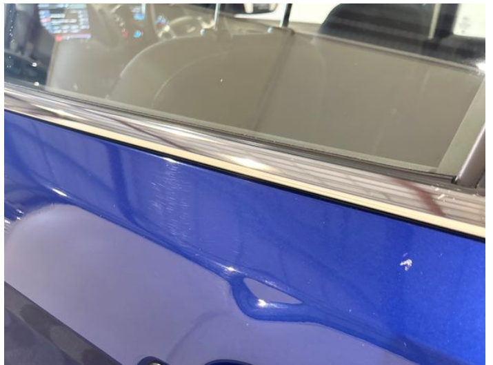
12: Door nsr Dented With Paint Damage
