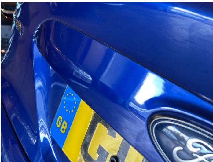
13: Tailgate Dented Between 10mm + 30mm
