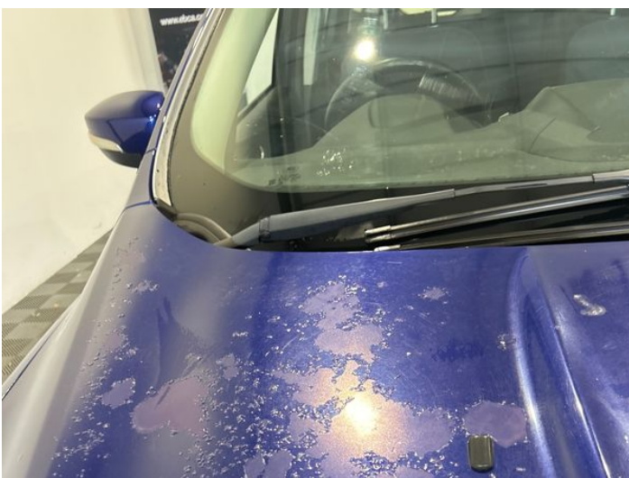
7: Bonnet Poor Previous Repair Paint Flake
