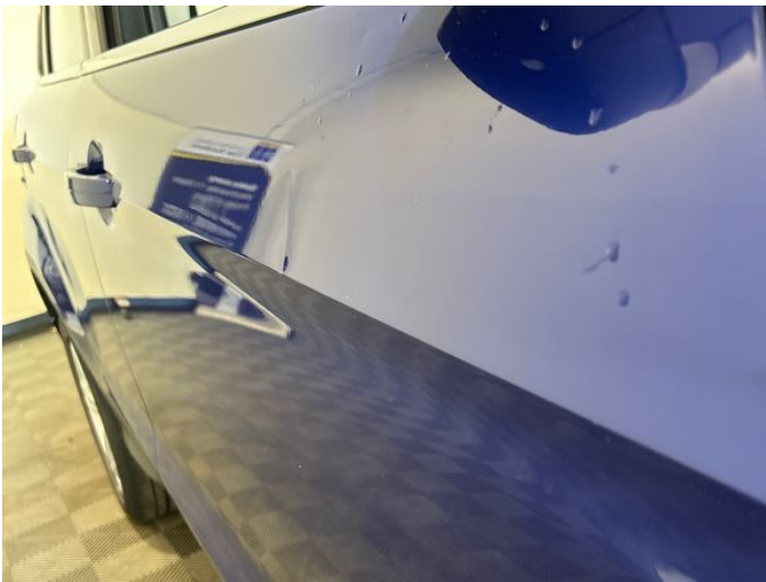
11: Door osf Dented Over 30mm
