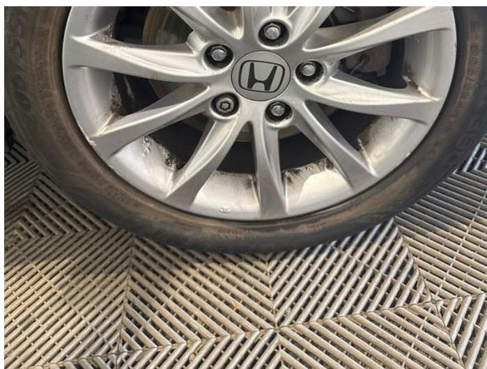
14: Wheel osf Scratched Over 50mm
