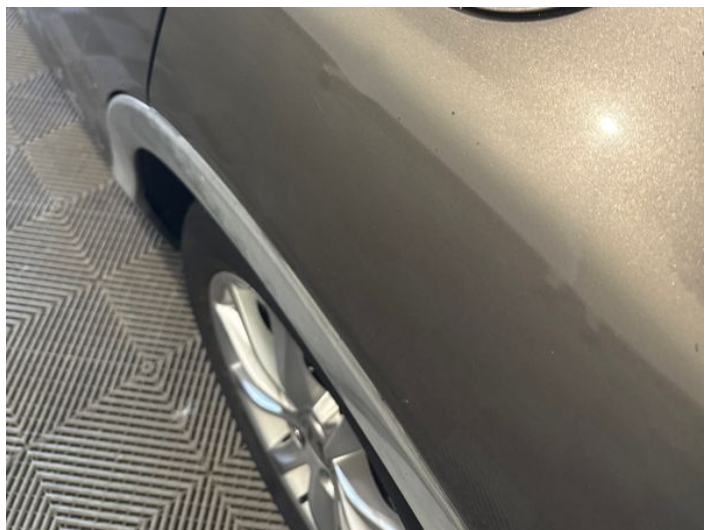
8: Qtr Panel nsr Dented Between 10mm + 30mm
