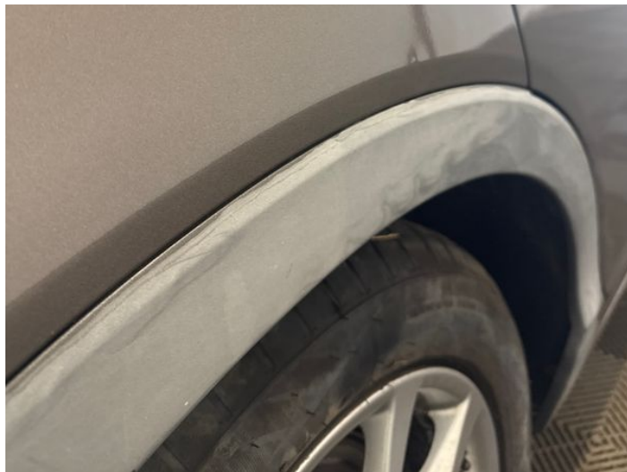
10: Qtr Panel osr Dented Between 10mm + 30mm
