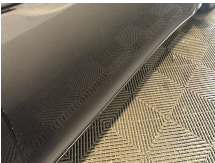
13: Door osf Dented With Paint Damage
