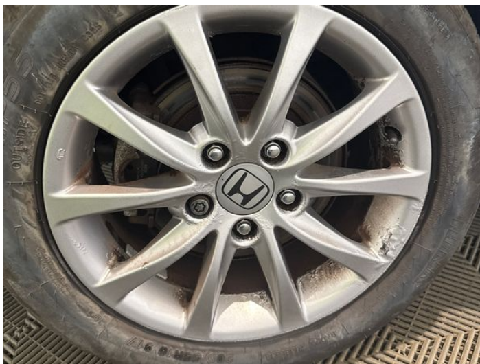
11: Wheel osr Scratched Over 50mm
