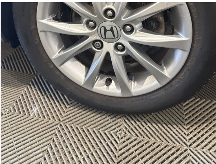
7: Wheel nsr Scratched Up To 50mm
