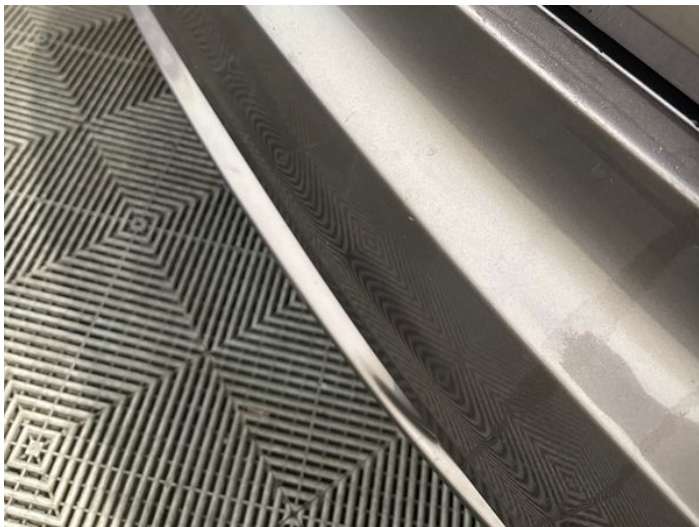
9: Bumper Rear Scratched 25 to 100mm Thru Paint
