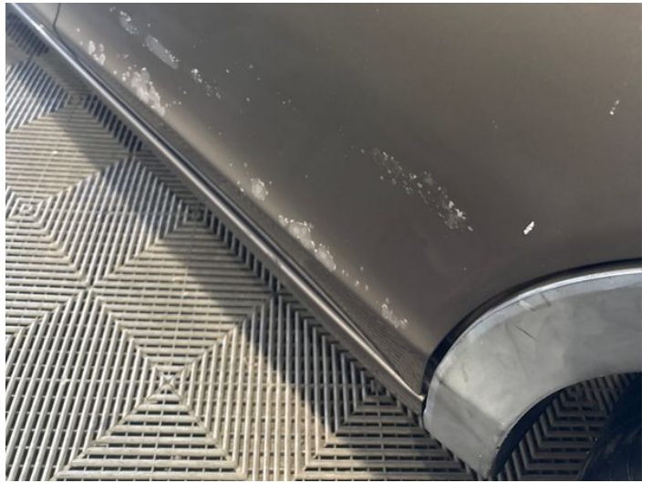
6: Door nsr Poor Previous Repair Paint Flake
