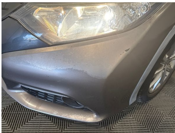
2: Bumper Front Dented With Paint Damage
