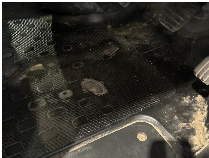
2: Carpets Front Holed Over 3mm
