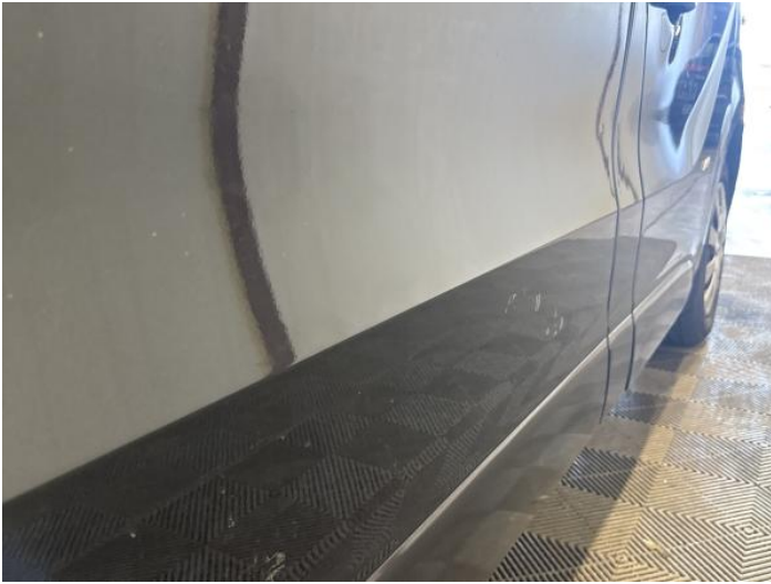
15: Panel Front Scratched Over 25mm Thru Paint
