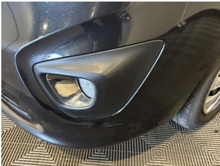
5: Bumper Front Scratched 25 to 100mm Thru Paint
