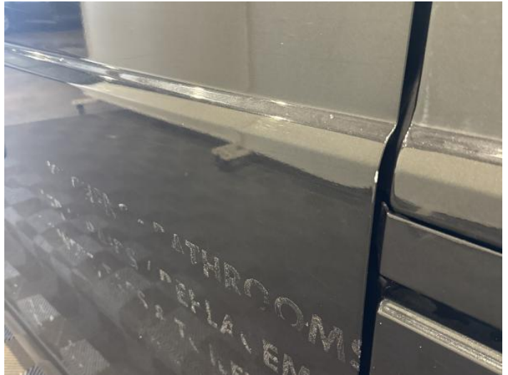
10: Door nsr Dented With Paint Damage
