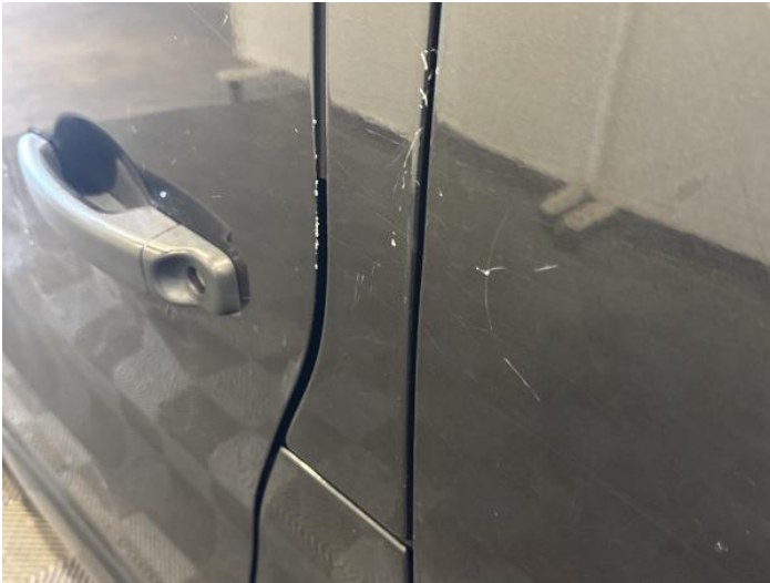
9: B Post ns Scratched Over 25mm Thru Paint
