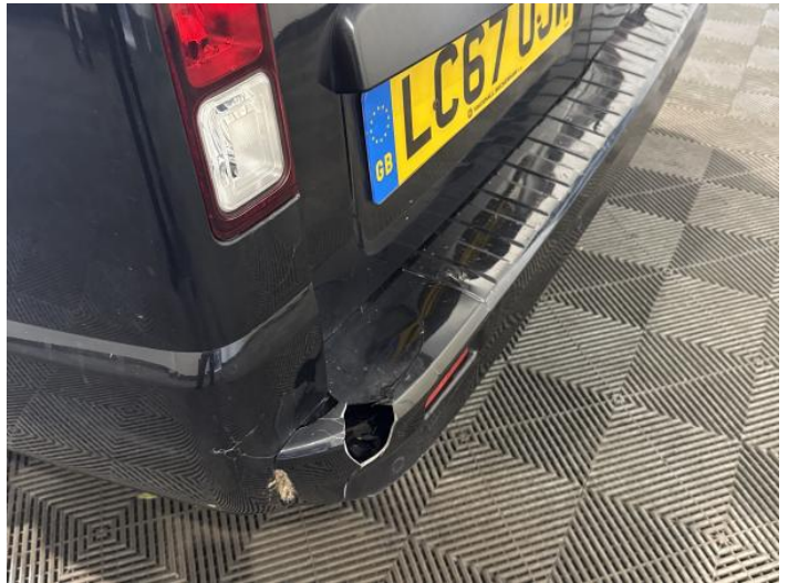
12: Bumper Rear Cracked Over 25mm
