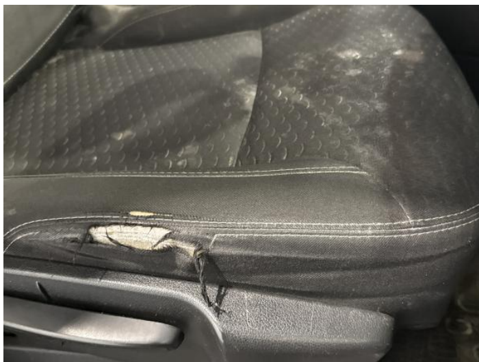
1: Seat Base Cover osf Torn Over 3mm
