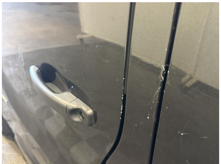
8: Door nsf Chipped Edge Chip
