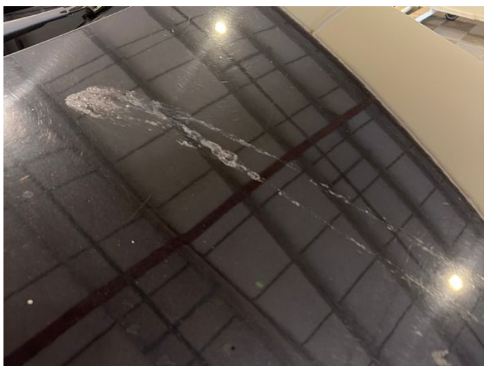
1: Bonnet Scratched Over 25mm Thru Paint
