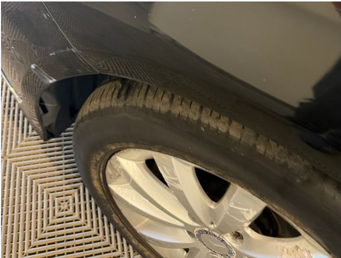
5: Wing nsf Scratched Over 25mm Thru Paint
