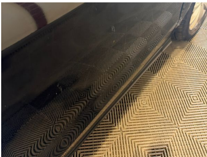
17: Door osf Scratched Over 25mm Thru Paint
