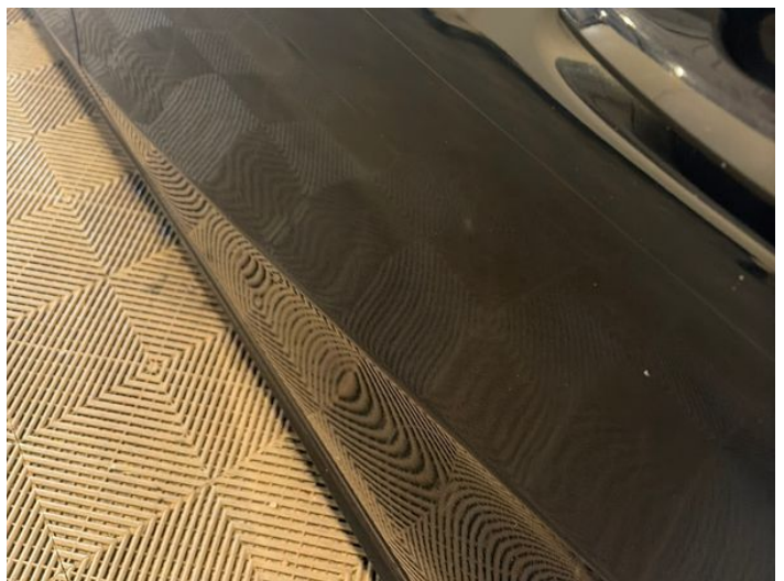
8: Door nsr Scratched Over 25mm Thru Paint
