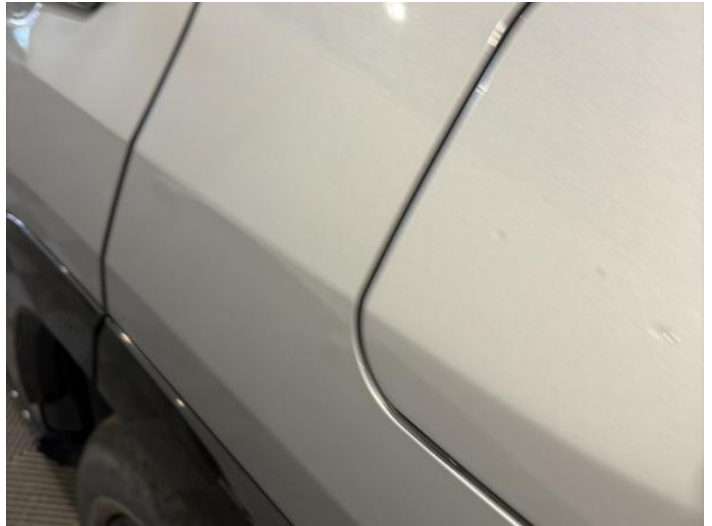
10: Qtr Panel nsr Dented Between 10mm + 30mm
