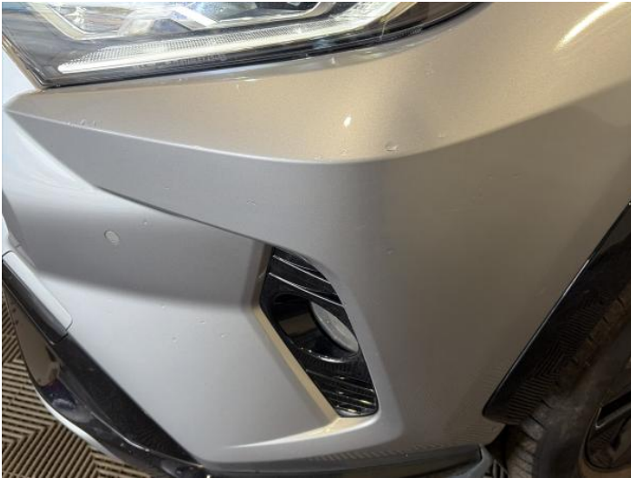
3: Bumper Front Scratched 25 to 100mm Thru Paint
