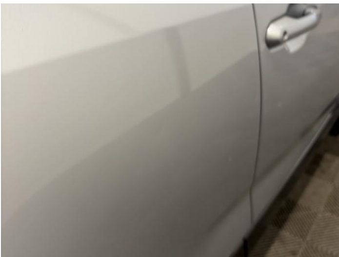
13: Door osr Dented Between 10mm + 30mm
