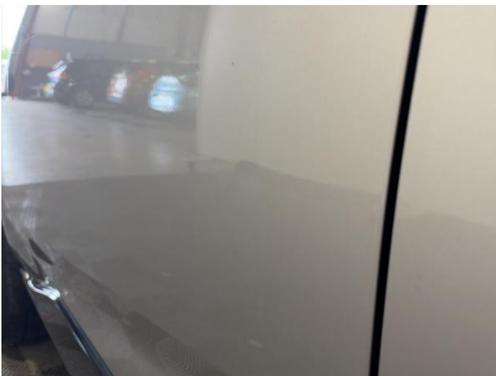
7: Door nsf Dented Between 10mm + 30mm
