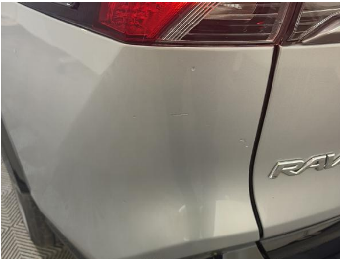
11: Bumper Rear Scratched Up To 25mm Thru Paint
