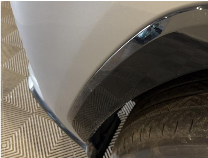
5: Wing Front Arch Extension ns Scratched (Painted) UpTo 25mm Thru Paint
