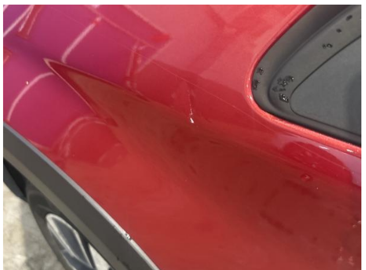
14: Wing nsf Dented With Paint Damage
