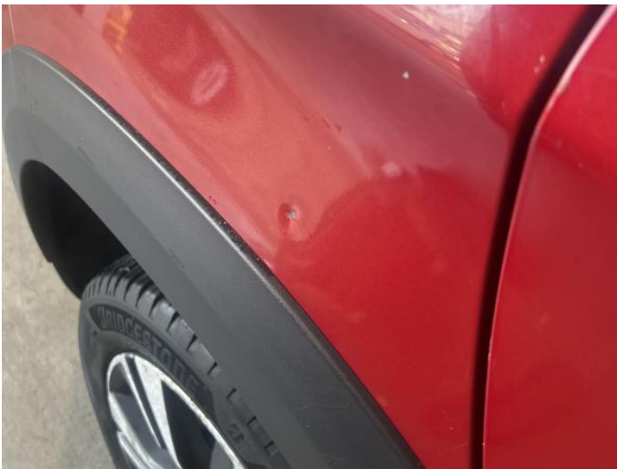
5: Qtr Panel osr Dented With Paint Damage
