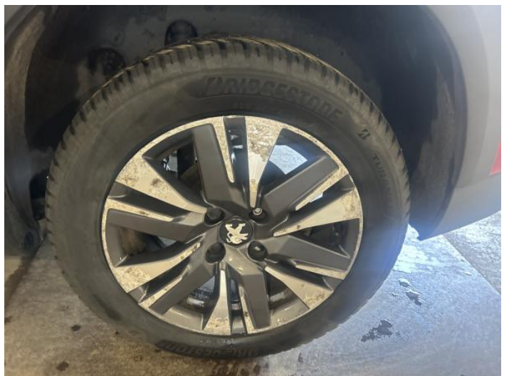
8: Wheel nsr Corroded Light
