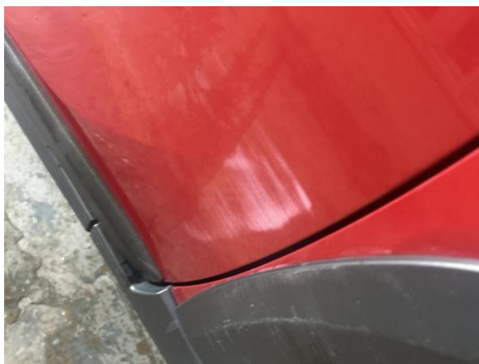
2: Door osf Scratched Over 25mm Thru Paint
