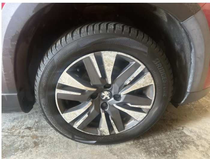
1: Wheel osf Corroded Light
