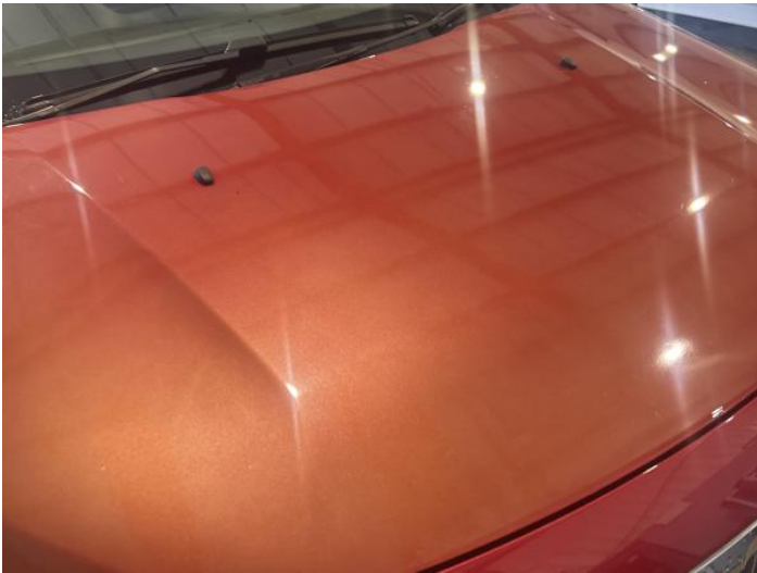
17: Bonnet Poor Previous Repair Poor Colour
