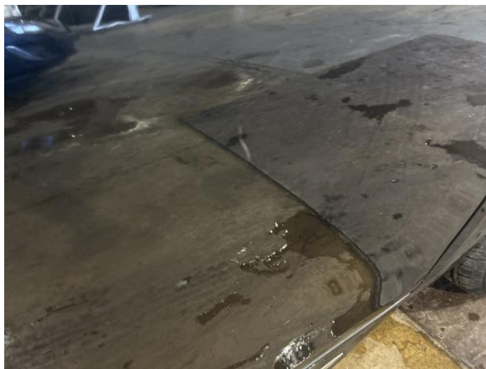
2: Door osf Scratched UpTo 25mm Thru Paint
