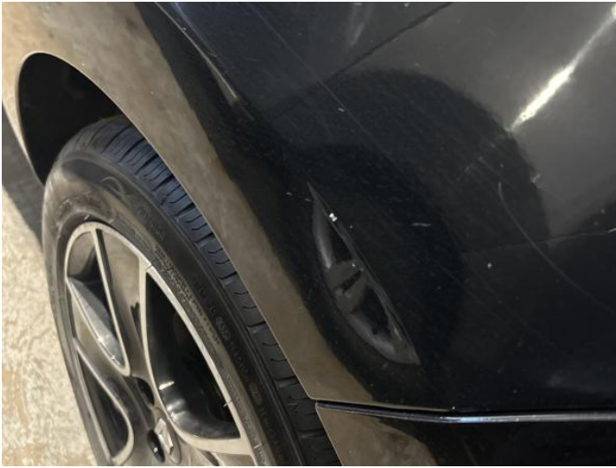
9: Qtr Panel nsr Chipped 1 To 5
