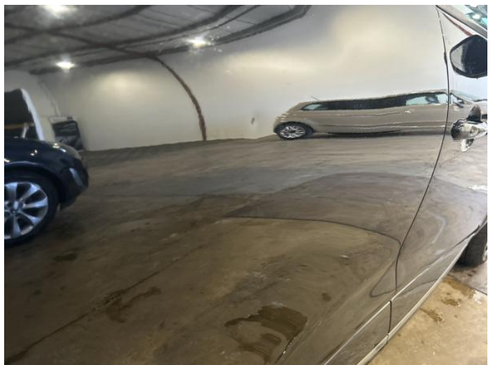
20: Door osr Dented 2 Or Less UpTo 10mm
