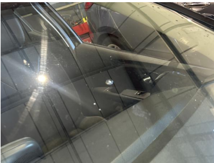
19: Screen Front Chipped UpTo 10mm
