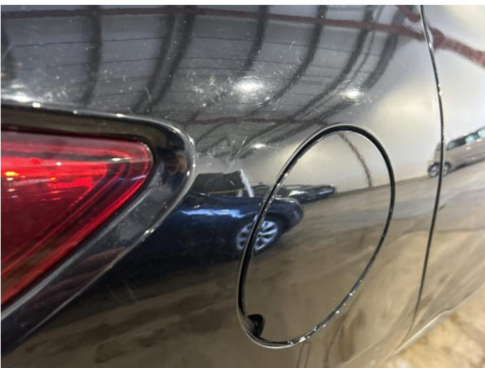
7: Qtr Panel osr Dented Between 10mm + 30mm
