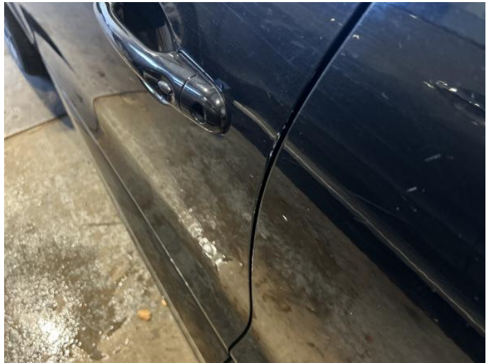
12: Door nsf Chipped Edge Chip
