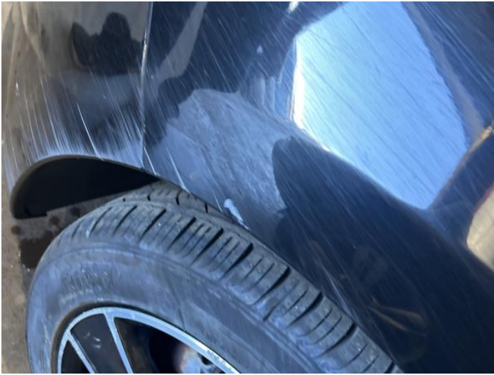
15: Wing nsf Scratched Over 25mm Thru Paint
