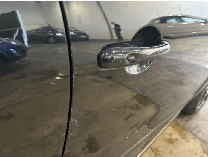
3: Door osf Chipped Edge Chip
