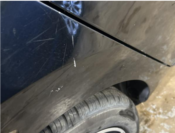
5: Qtr Panel osr Chipped 1 To 5
