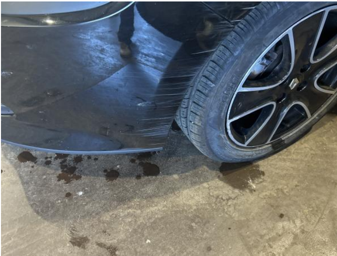
17: Bumper Front Scratched 25 to 100mm Thru Paint
