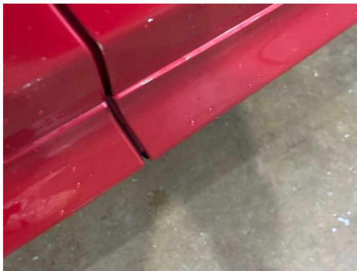
2: Door osf Chipped 1 To 5
