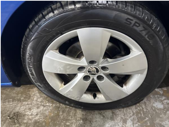
18: Wheel osf Scratched Up To 50mm
