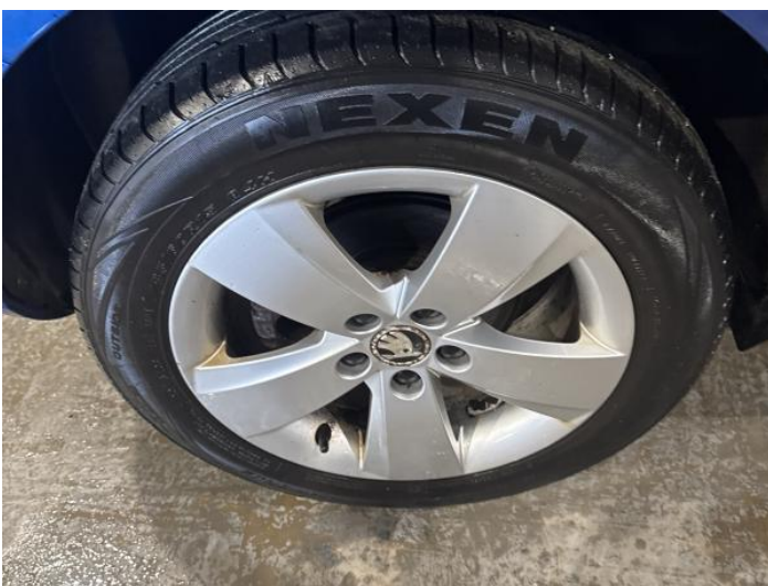
13: Wheel osr Scratched Up To 50mm
