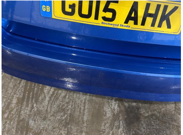
10: Bumper Rear Chipped Multiple Chips
