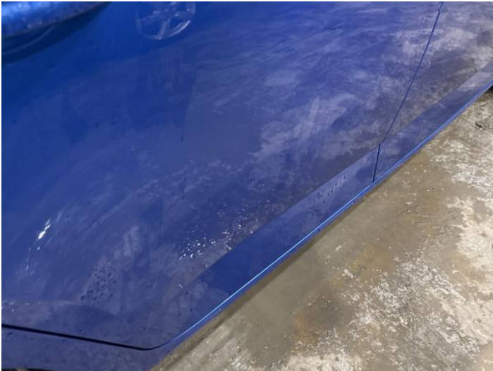
15: Door osr Scratched Over 25mm Not Thru Paint
