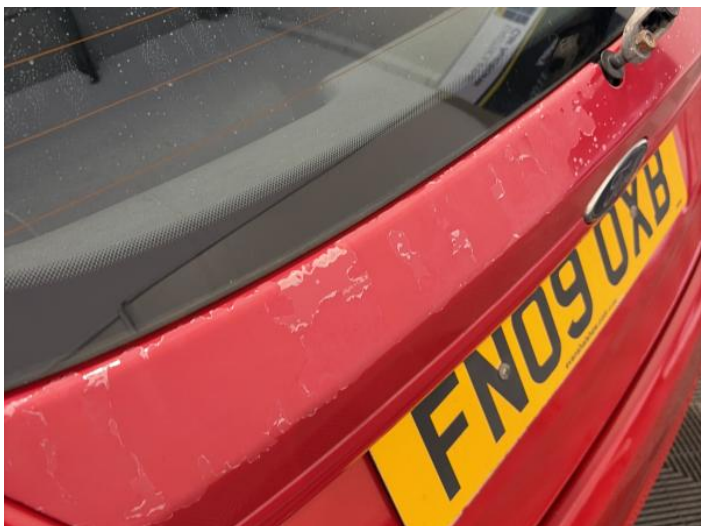
9: Tailgate Poor Previous Repair Paint Flake
