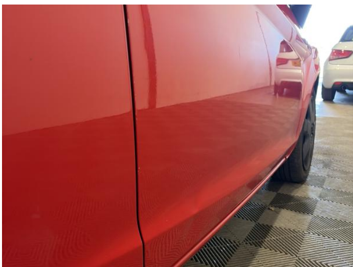
13: Door osf Dented Over 30mm
