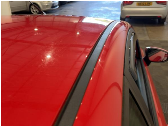
15: Roof Dented Over 30mm
