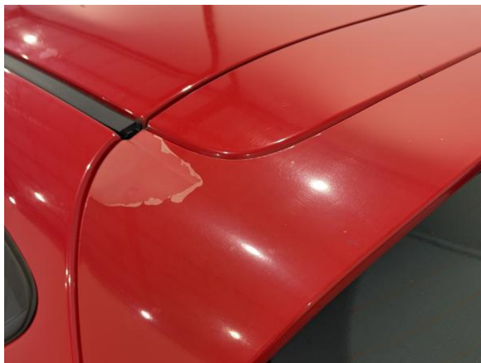
10: Spoiler Rear Scratched (Painted) Over 25mm Thru Paint
