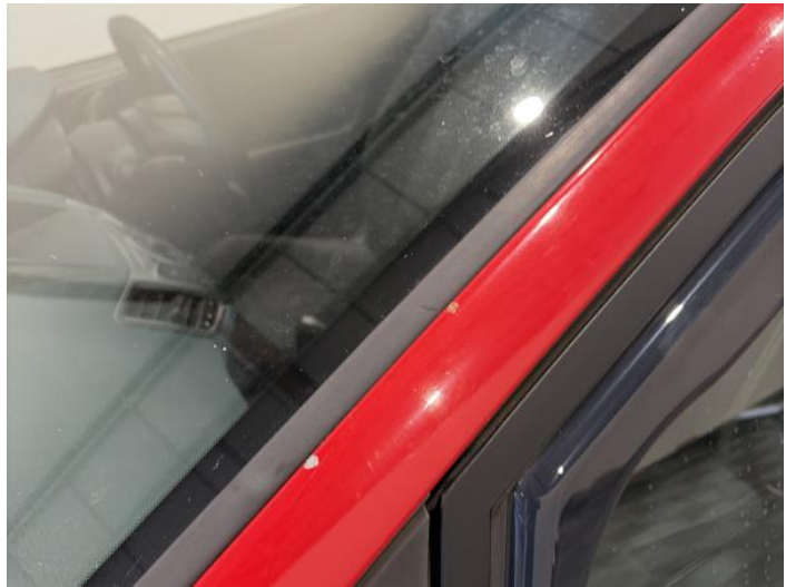
6: A Post ns Chipped Over 5mm
