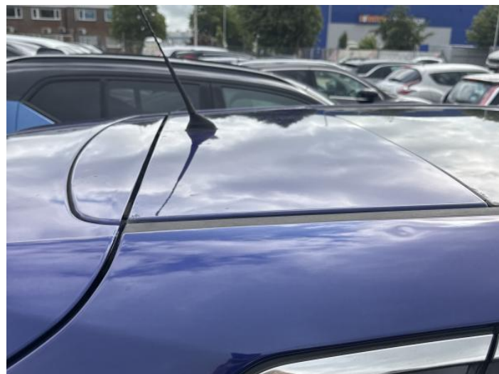
25: Roof Dented Hail - Moderate
